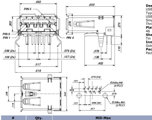
**Description: USB** Socket Type A **USB 3.0** Single Row Through Hole Plating Code: Shell Plating: Tin Plated **Inner Contact Plating:**
