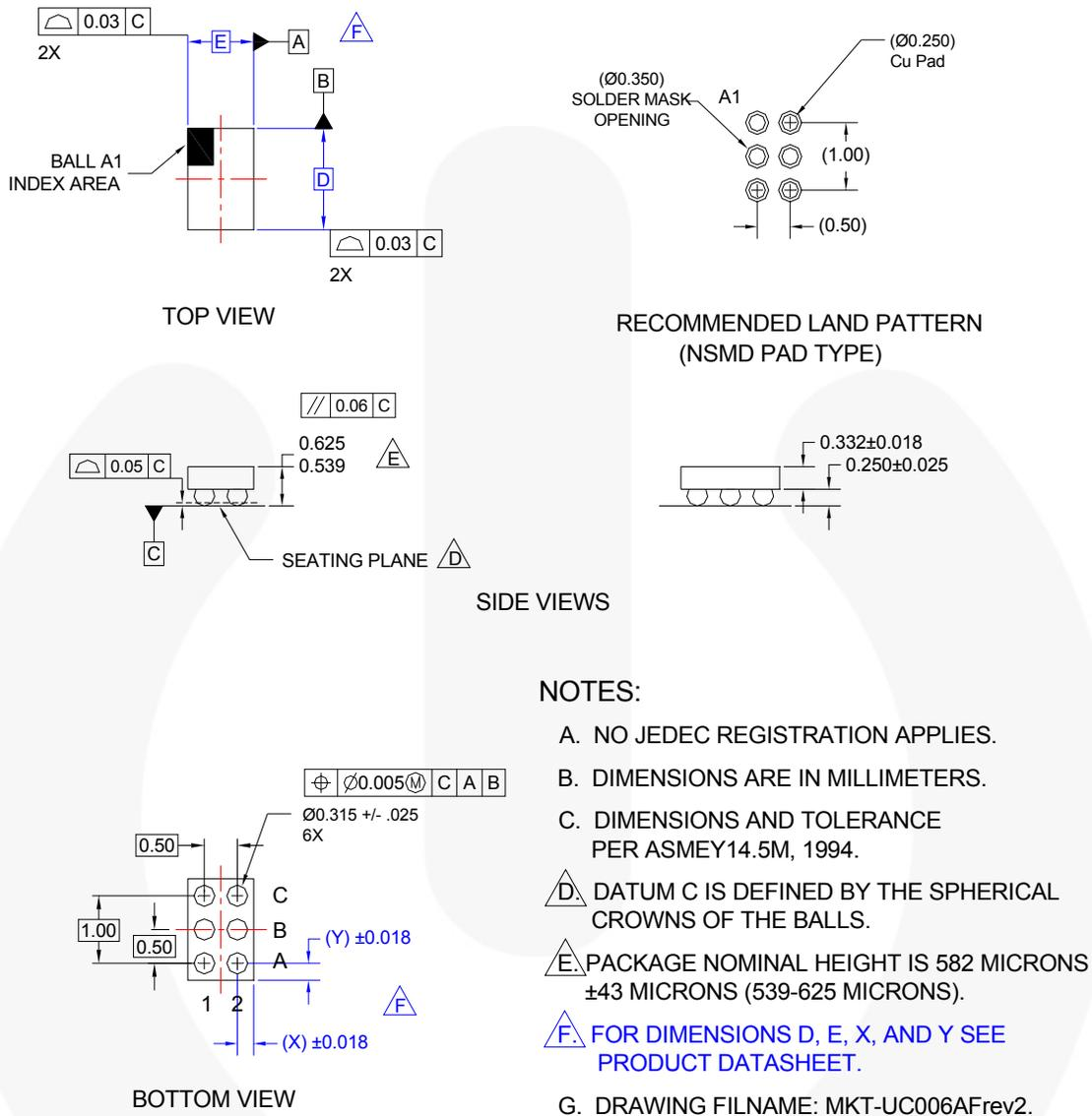
Figure 29. 6-Ball WLCSP, 2x3 Array, 0.5mm Pitch, 300µm Ball
