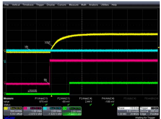
FIGURE 16. POWER-ON AND POWER-OFF, EN = 0 TO 1 , +25^\circ C , V_{IN} = 2.2V , V_{OUT} = 0.8V , I_{OUT} = 0.5A , PGOOD TURN-ON
