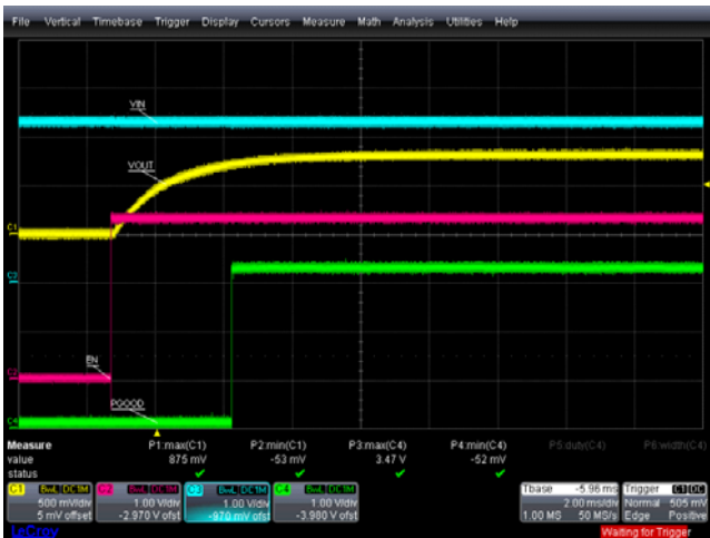
FIGURE 15. POWER-ON AND POWER-OFF, EN = 0 TO 1 , +25^\circ C , V_{IN} = 6V , V_{OUT} = 0.8V , I_{OUT} = 0.5A , PGOOD TURN-ON
