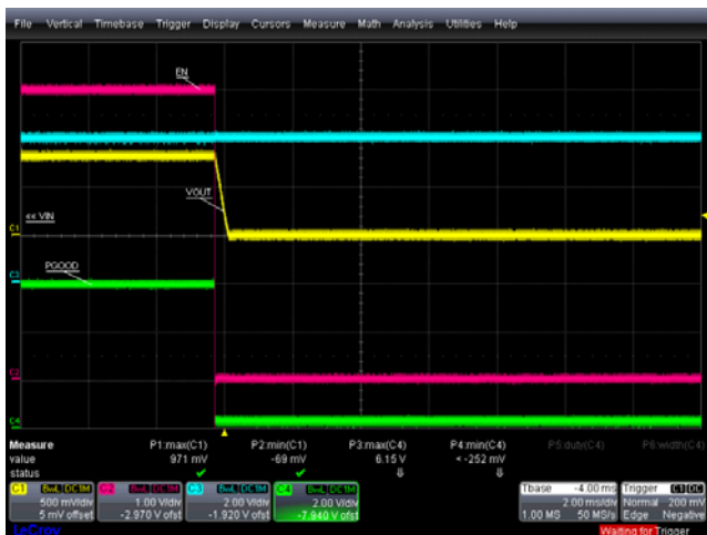
FIGURE 17. POWER-ON AND POWER-OFF, EN = 1 TO 0 , +25^\circ C , V_{IN} = 6V , V_{OUT} = 0.8V , I_{OUT} = 0.5A , PGOOD TURN-OFF
