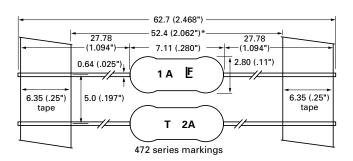
Coating Diameter (max): 0.5A-3.0A: 2.80mm 5.0A: 2.90mm
