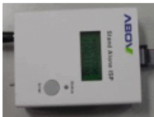
Figure 1-3 StandAlone ISP (VDD power is not supplied)
