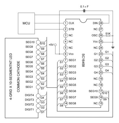
Note: the capacitor (0.1 $\mu$ F) connected between the GND and VDD pins must be located as near as possible to the SC16458 chip.
