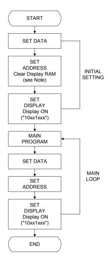
Note: When IC power is applied for the first time, the contents of the display RAM are not defined; thus, it is strongly suggested that the contents of the display RAM must be cleared during the initial setting.
