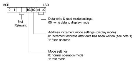
Note: 1. If you want to set bit 3 (b2) to "0", please remember that DIG5 address cannot be ignored since G5 exists, however, it is not externally bonded. Please refer to command 2, display mode and RAM address section.
