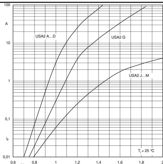
Fig. 1 Forward characteristics (typical values)
