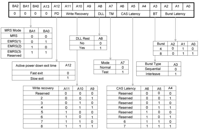
Note1. Active power down exit time's fast exit (A12=0) use t<sub>XARD</sub> and slow exit (A12=1) use t<sub>XARDS</sub>.
