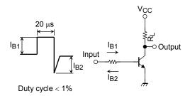
Figure 1 Switching Time Test Circuit & Timing Chart
