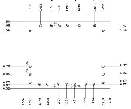
Units: millimeters Thickness: 0.380
