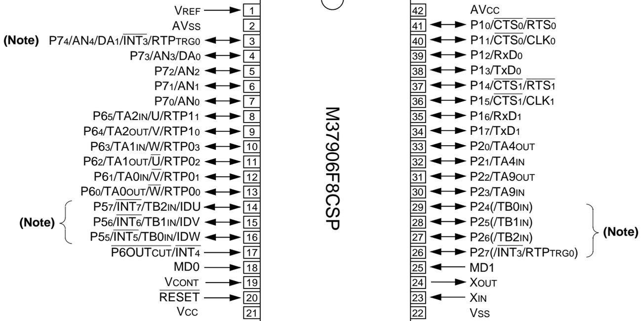
**Note:** Allocation of pins TB0IN to TB2IN and INT3/RTPTRG0 can be switched by software.
