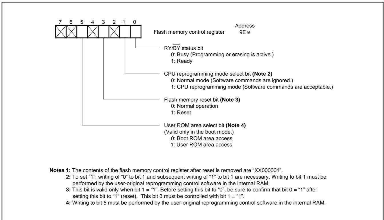
Fig. 7 Bit configuration of flash memory control register
