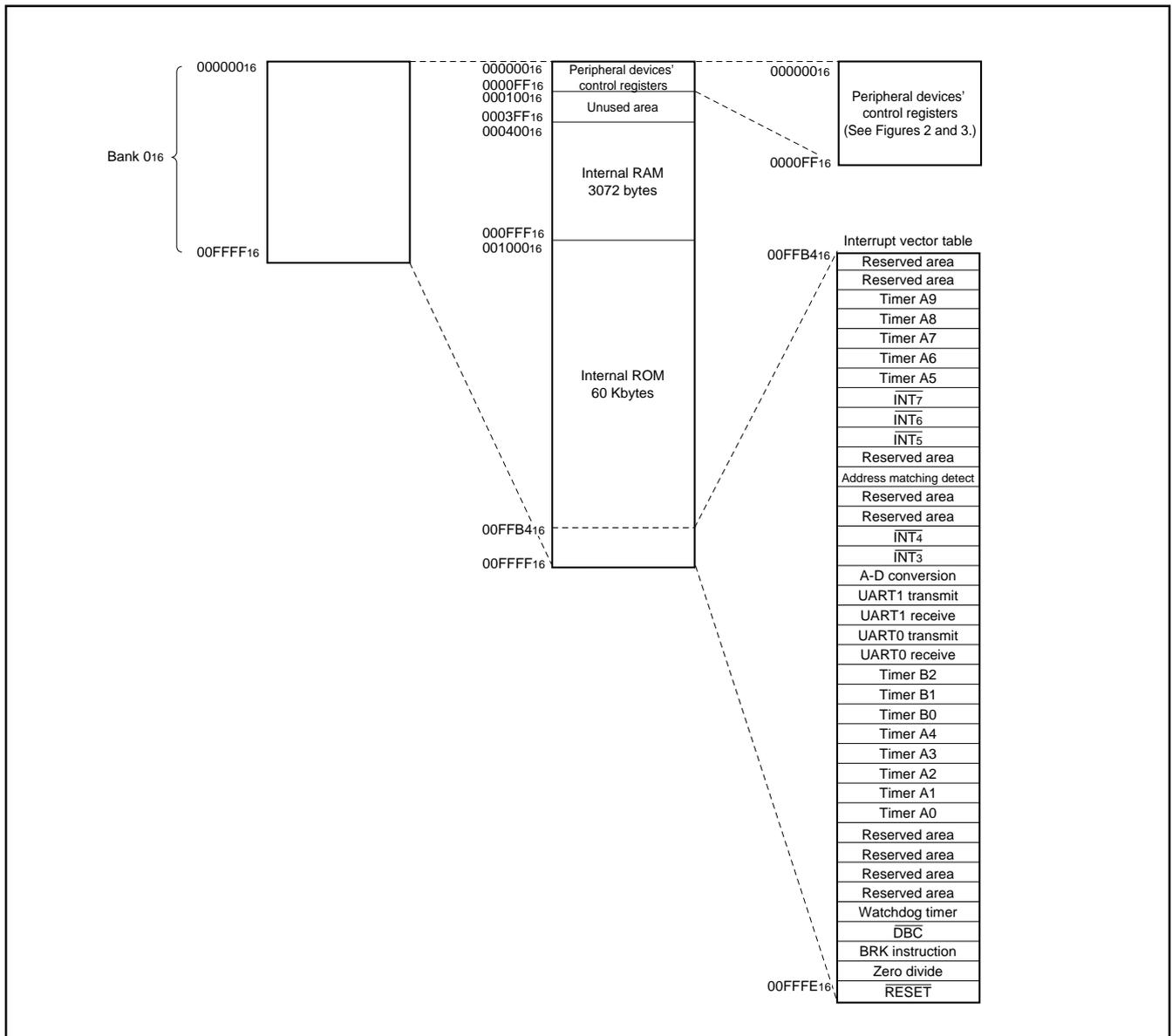
Fig. 1 Memory map of M37906F8CFP, M37906F8CSP (Single-chip mode)
