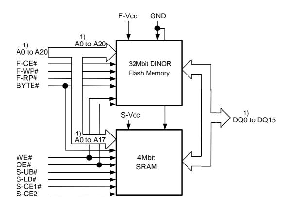
Note 1): In case of x8 organization, A-1 is added, and only Lower Byte data(DQ0 to DQ7) are assigned to I/O and Upper Byte data(DQ8 to DQ15) are High-Z.
