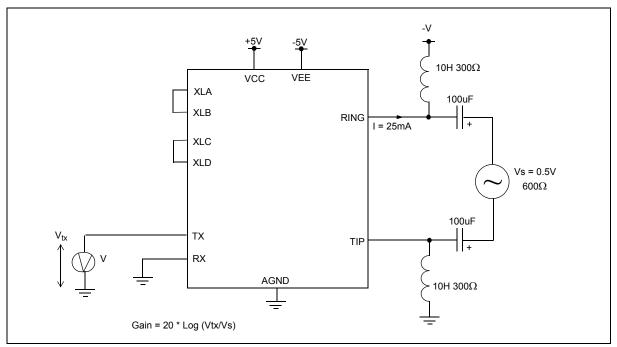
Figure 4 - 2-4 Wire Gain Test Circuit
