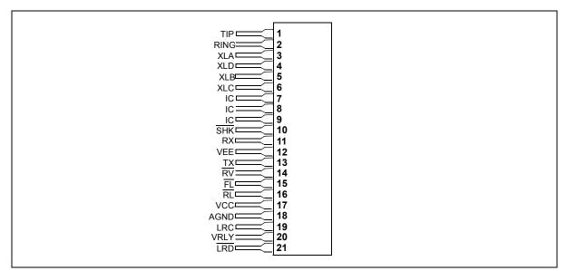
Figure 2 - Pin Connections
