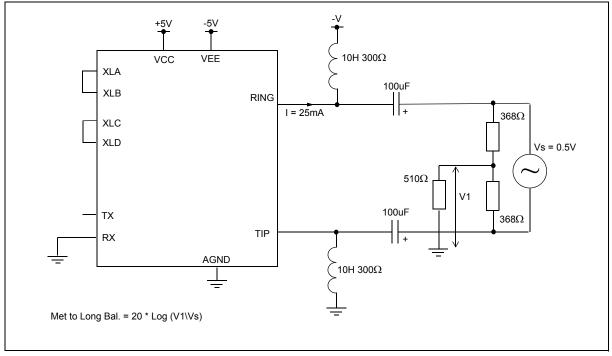
Figure 8 - Metallic to Longitudinal Balance Test Circuit
