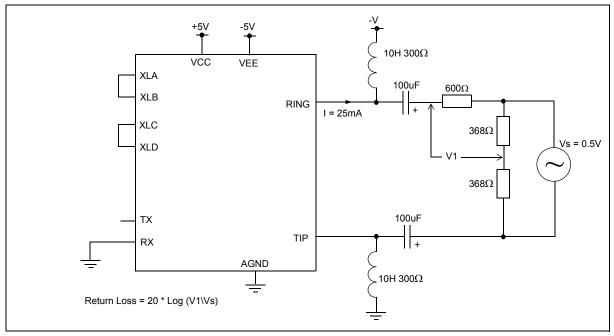
Figure 6 - Return Loss Test Circuit
