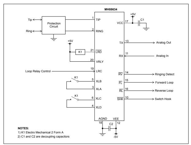
Figure 3 - Typical LS Application Circuit
