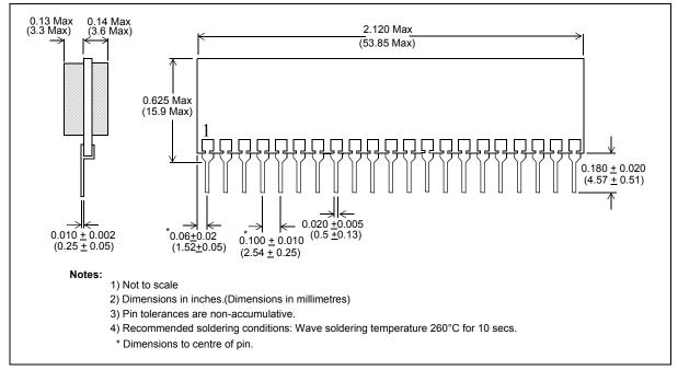
Figure 9 - Mechanical Data (SIL Package)
