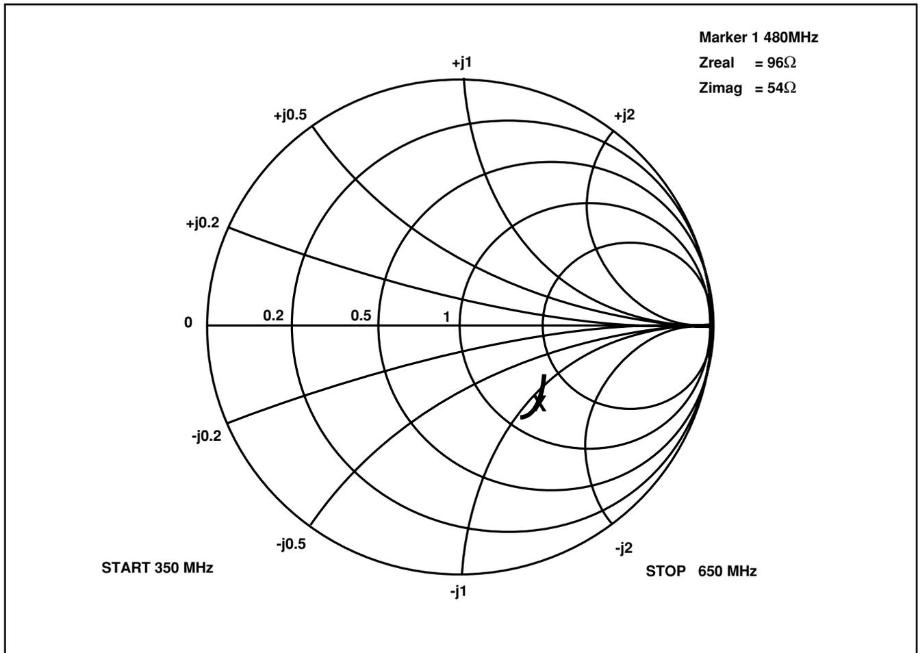
Fig.3 Typical RF input impedance
