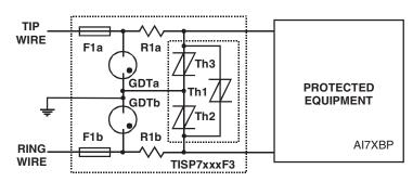
Figure 36. Protection Module
