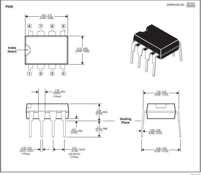
NOTES: A. Each pin centerline is located within 0.25 (0.010) of its true longitudinal position. B. Dimensions fall within JEDEC MS001 - R-PDIP-T, 0.300" Dual-In-Line Plastic Family. MDXXCF
