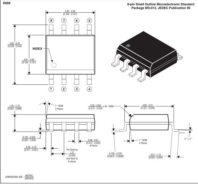
NOTES: A. Leads are within 0.25 (0.010) radius of true position at maximum material condition.
