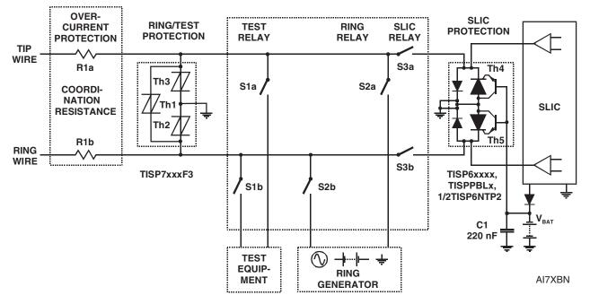
Figure 38. Line Card Ring/Test Protection
