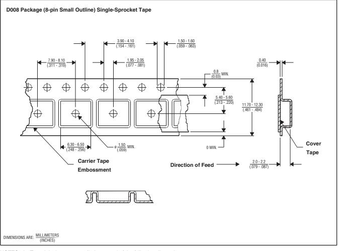
NOTES: A. Taped devices are supplied on a reel of the following dimensions:-
