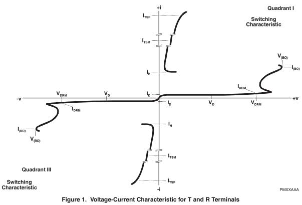
T and G and R and G Measurements are Referenced to the G Terminal T and R Measurements are Referenced to the R Terminal
