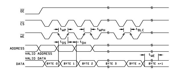
FIGURE 6. Page write timing diagram.
