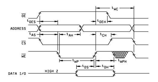
FIGURE 5. Write cycle timing diagram - WE controlled.
