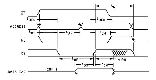
FIGURE 5. Write cycle timing diagram - CS controlled.
