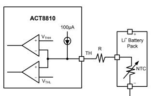
at low temperatures by connecting a resistor in parallel with I<sub>TH</sub>. The desired resistance can be found using the following equation:  $(I_{TH} + (V_{CHG IN} - V_{THL})/R) \times k_{COLD} @0^{\circ}C) \times R_{NOM} = V_{THL}$
