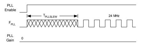
Figure 7. PLL Lock for Low Gain Setting Timing Diagram
