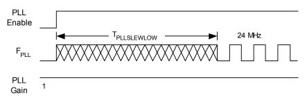
Figure 8. External Crystal Oscillator Startup Timing Diagram
