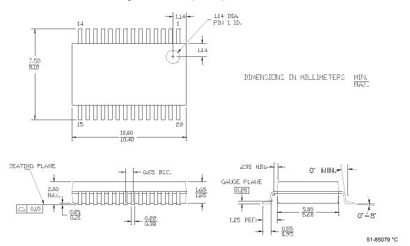
Figure 16. 28-Pin (210-Mil) SSOP
