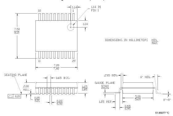
Figure 15. 20-Pin (210-Mil) SSOP
