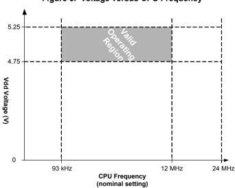
Figure 5. Voltage versus CPU Frequency
