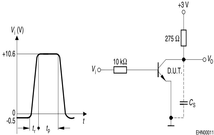
Input waveform;  $t_r < 1ns$ ;  $t_p = 300$  ns
