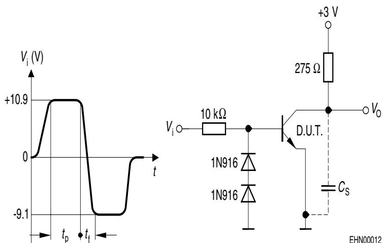
Input waveform;  $t_r < 1ns$ ;  $10 \mu s < t_p \leq 500 \mu s$
