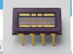
S9226 is a small CMOS linear image sensor designed for image input applications. The signal processing circuit has a charge amplifier with excellent input/output characteristics.
