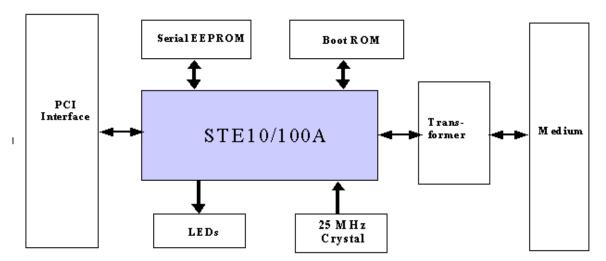
The STE10/100A provides both half-duplex and full-duplex operation, as well as support for full-duplex flow control. It provides long FIFO buffers for transmission and receiving, and early interrupt mechanism to enhance performance. The STE10/100A also supports ACPI and PCI compliant power management functions. Some key features are listed as follows:
