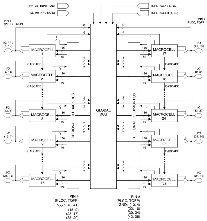
Note: 1. Arrows connecting macrocells indicate direction and groupings of CASIN/CASOUT data flow.
