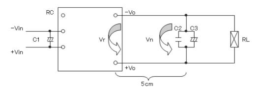
Vr: Testing point of output voltage, output regulation.
