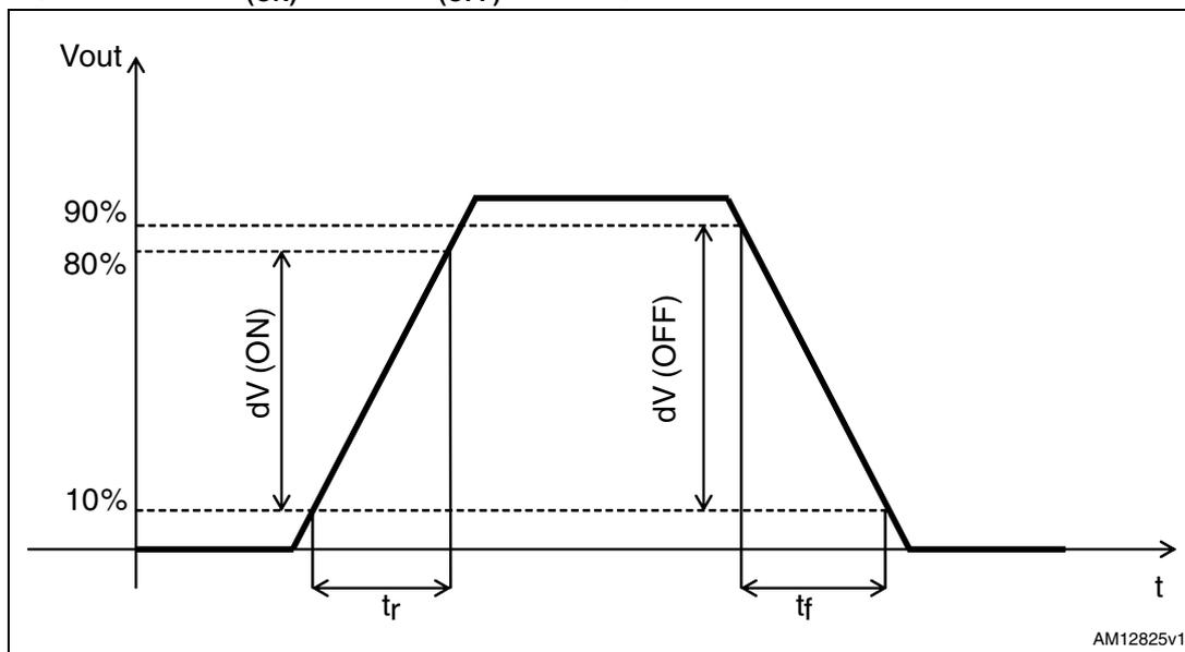
Figure 15.  $t_{d(ON)}$  and  $t_{d(OFF)}$  time diagram test conditions
