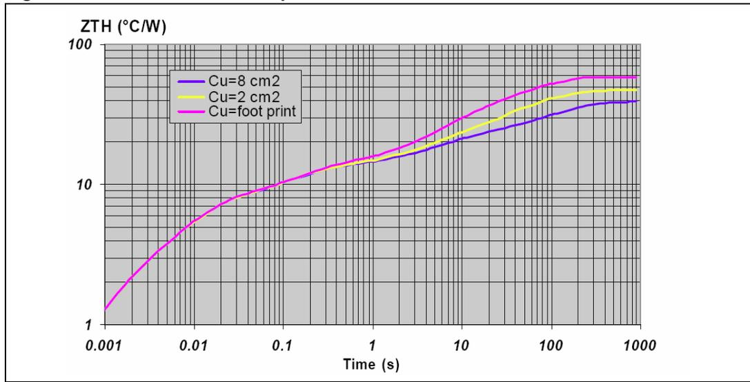
For instance, three cases have been considered using a PSSO36 packaged with copper slug soldered on a 1.6 mm thickness FR4 board with dissipating footprint (copper thickness of 70  $\mu\text{m}$ ):
