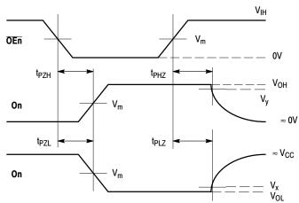
WAVEFORM 3 - PROPAGATION DELAYS  $t_{R}$  =  $t_{F}$  = 2.0 ns, 10% to 90%; f = 1 MHz;  $t_{W}$  = 500 ns
