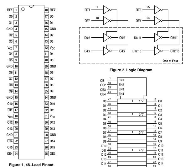
Figure 1. 48–Lead Pinout (Top View)
