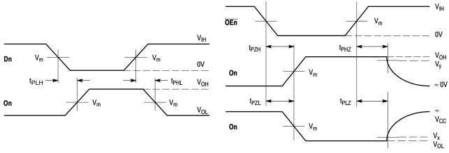
**WAVEFORM 1 - PROPAGATION DELAYS**  $t_{R} = t_{F} = 2.0$  ns, 10% to 90%; f = 1 MHz;  $t_{W} = 500$  ns WAVEFORM 2 - OUTPUT ENABLE AND DISABLE TIMES  $t_R$  =  $t_F$  = 2.0 ns, 10% to 90%; f = 1 MHz;  $t_W$  = 500 ns
