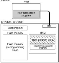
2. Programming control program transfer When boot mode is entered, the boot program in the SH7052F, SH7053F (originally incorporated in the chip) is started and the programming control program in the host is transferred to RAM via SCI communication. The boot program required for flash memory erasing is automatically transferred to the RAM boot program area.
