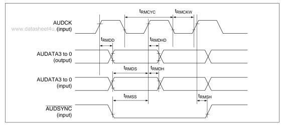
Figure 24.22 RAM Monitor Mode Timing
