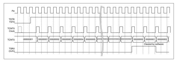
Figure 10.13 Free-Running Counter Operation and Overflow Timing
