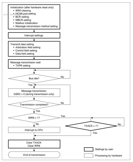
Figure 15.7 Transmission Flowchart
