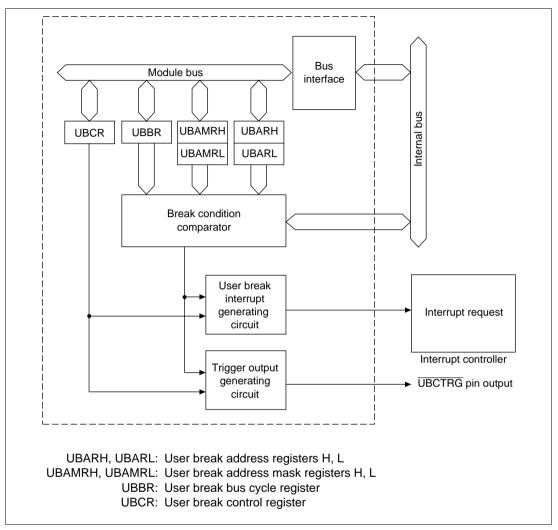
Figure 7.1 User Break Controller Block Diagram
