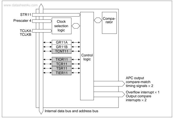
Figure 10.10 Block Diagram of Channel 11
