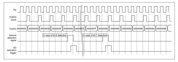
Figure 10.19 Interval Timer Function
