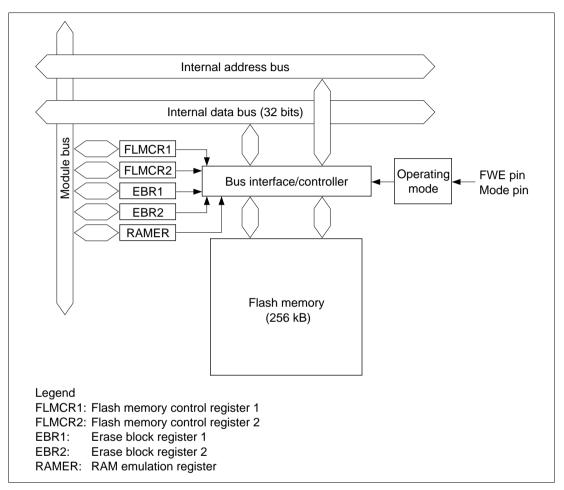
Figure 20.1 Block Diagram of Flash Memory
