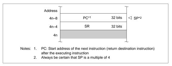
Figure 6.3 Stack after Interrupt Exception Processing
