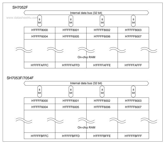
Figure 22.1 Block Diagram of RAM
