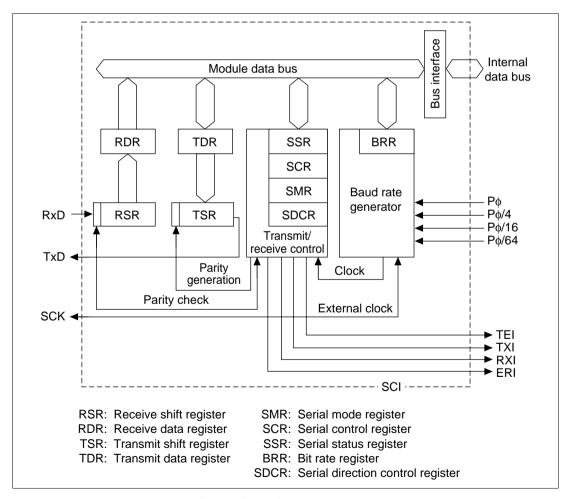
Figure 14.1 SCI Block Diagram WWW.DataSheet4U.com
