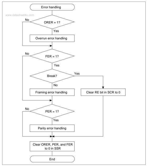
Figure 14.8 Sample Flowchart for Receiving Serial Data (2)
