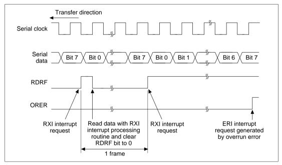
Figure 14.23 Example of SCI Receive Operation
