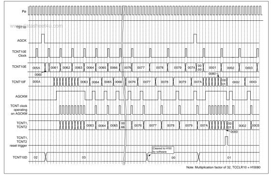
Figure 10.35 TCNT10F Operation (End of Cycle, Acceleration, Deceleration)
