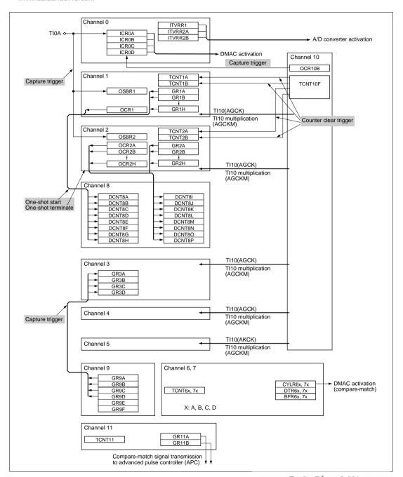
Figure 10.11 Inter-Module Communication Signata Sheet 4U.com
