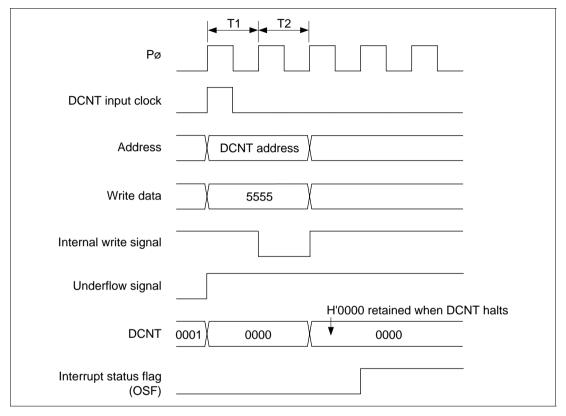
Figure 10.72 Contention between DCNT Write and Underflow
