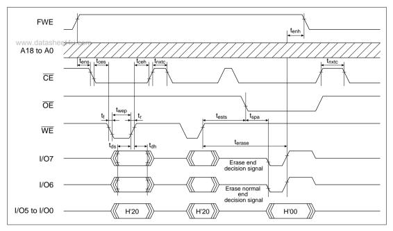
Figure 20.26 Auto-Erase Mode Timing Waveforms
