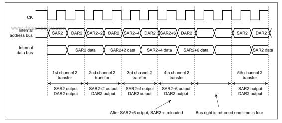
Figure 9.11 Source Address Reload Function Timing Chart
