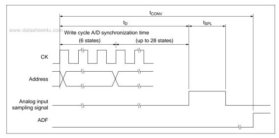
Figure 24.19 Analog Conversion Timing
