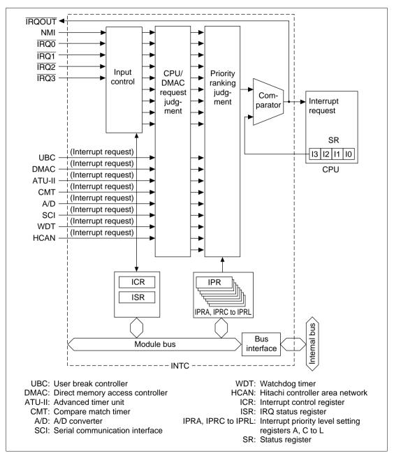
Figure 6.1 INTC Block Diagram
