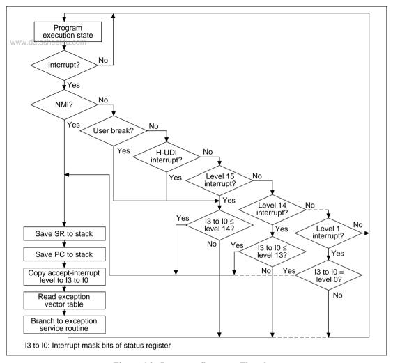
Figure 6.2 Interrupt Sequence Flowchart
