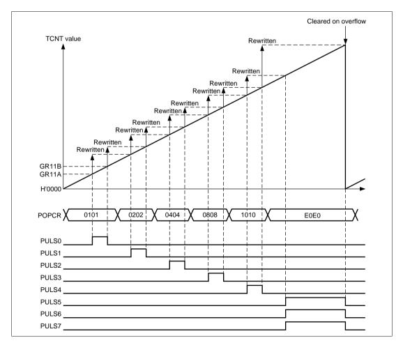
Figure 11.4 Example of Advanced Pulse Controller Quiput Operation 411 com
