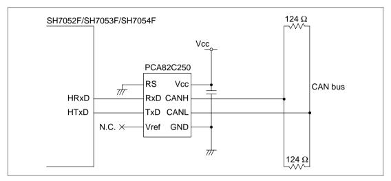
Figure 15.14 Example of High-Speed Interface Using PCA82C250
