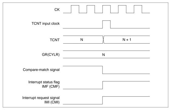
Figure 10.38 IMF (CMF) Setting Timing in Compare-Match
