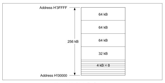
Figure 20.7 Block Configuration
