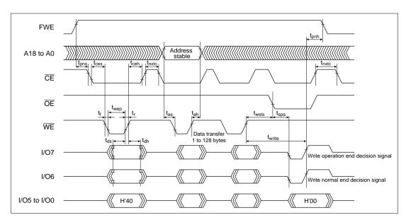
Figure 20.25 Auto-Program Mode Timing Waveforms
