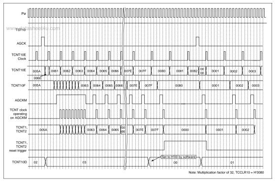
Figure 10.36 TCNT10F Operation (End of Cycle, Steady-State)
