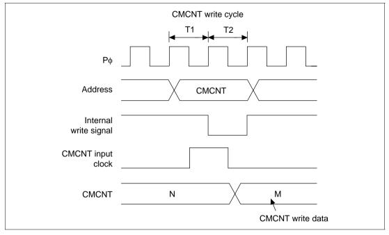
Figure 13.7 CMCNT Word Write and Increment Contention
