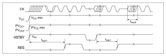
Figure 24.4 Oscillation Settling Time
