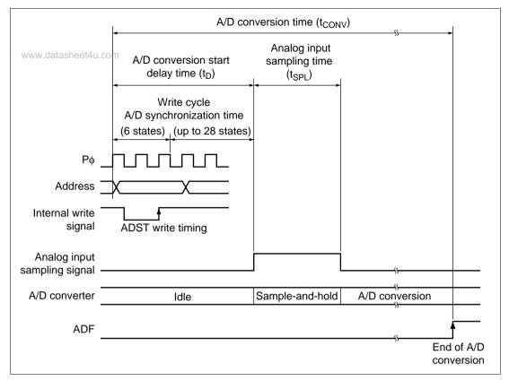
Figure 16.6 A/D Conversion Timing
