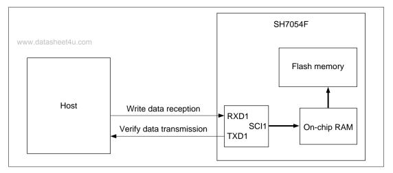
Figure 21.8 System Configuration in Boot Mode
