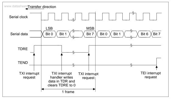
Figure 14.20 Example of SCI Transmit Operation
