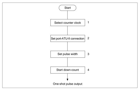
Figure 10.56 Sample Setup Procedure for One-Shot Pulse Output
