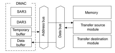
The value in the temporary buffer is taken as the address, and data is read from the transfer source module to the data buffer.
