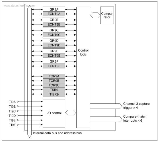
Figure 10.8 Block Diagram of Channel 9
