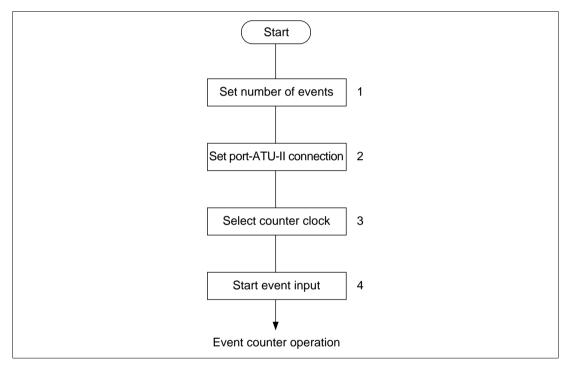
Figure 10.61 Sample Setup Procedure for Event Counter Operation
