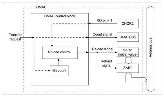
Figure 9.10 Source Address Reload Function
