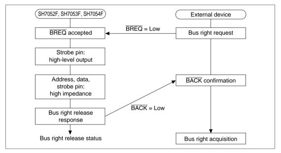
Figure 8.9 Bus Right Release Procedure
