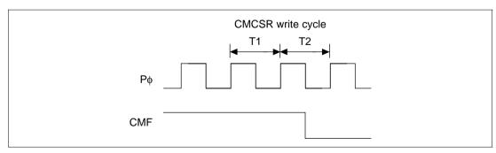
Figure 13.5 Timing of CMF Clear by the CPU
