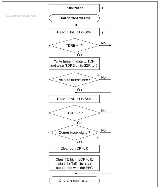
Figure 14.5 Sample Flowchart for Transmitting Serial Data
