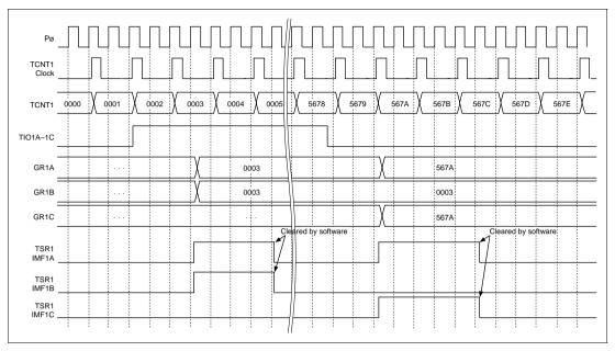
Figure 10.16 Input Capture Operation
