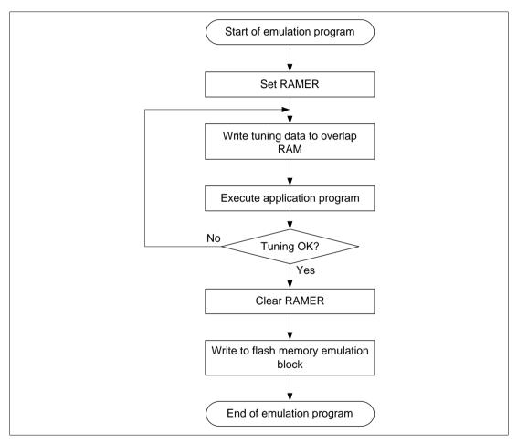
$Figure\ 21.17\quad Flowchart\ for\ Flash\ Memory\ Emulation\ in\ RAM$
