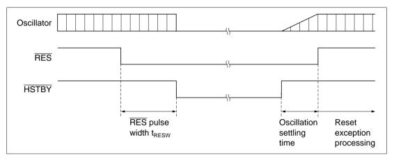
Figure 23.2 Hardware Standby Mode Timing
