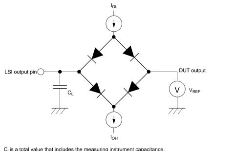
C<sub>L</sub> is a total value that includes the measuring instrument capacitance.
