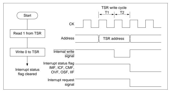
Figure 10.42 Procedure and Timing for Clearing by CPU Program
