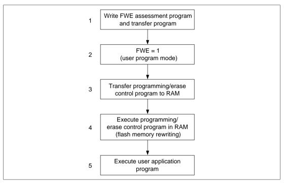
Figure 21.12 User Program Mode Execution Procedure
