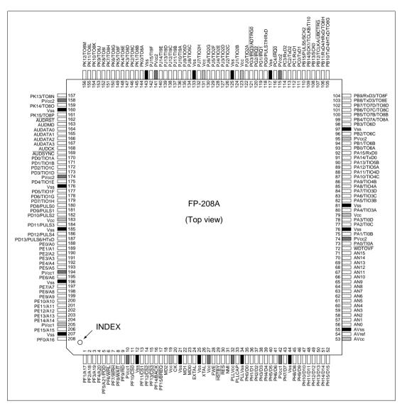
Figure 1.2 Pin Arrangement
