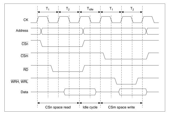
Figure 8.7 Idle Cycle Insertion Example www.DataSheet4U.com
