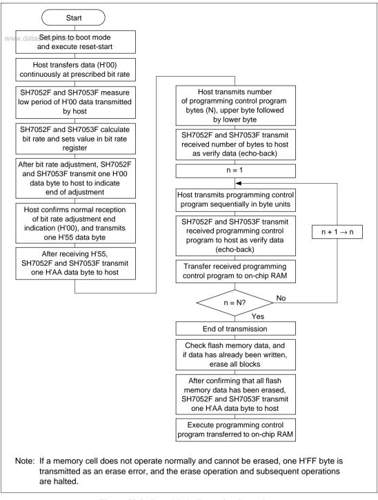
Figure 20.9 Boot Mode Execution Procedure
