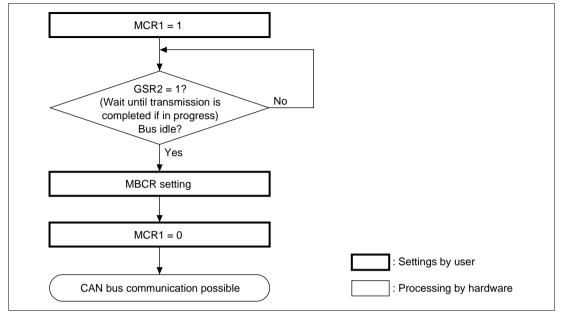
Figure 15.12 HCAN Halt Mode Flowchart
