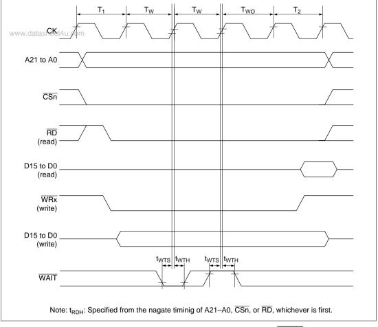
Figure 24.10 Basic Cycle (Two Software Waits + Waits by WAIT Signal)
