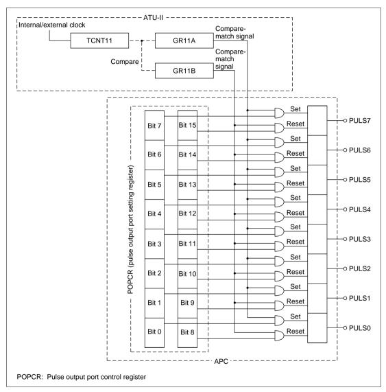
Figure 11.1 Advanced Pulse Controller Block Diagram
