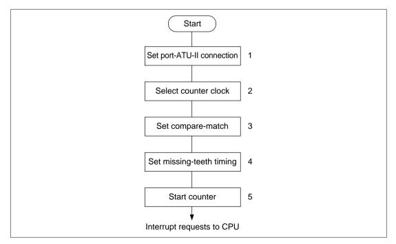
Figure 10.63 Sample Setup Procedure for Missing Teeth Detection 4U.com
