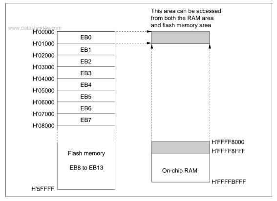
Figure 21.18 Example of RAM Overlap Operation
