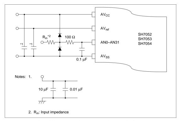
Figure 16.8 Example of Analog Input Pin Protection Circuit
