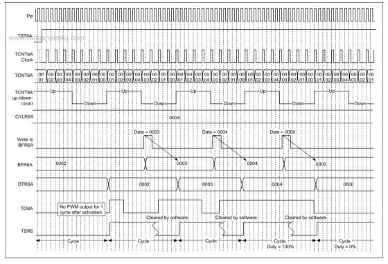
Figure 10.22 Complementary PWM Mode Operation
