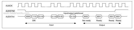
Figure 17.6 Example of Write Operation (Longword Read)
