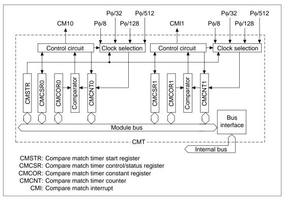
Figure 13.1 CMT Block Diagram
