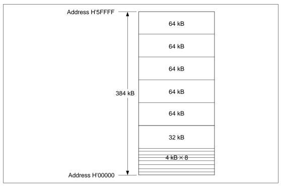
Figure 21.7 Block Configuration
