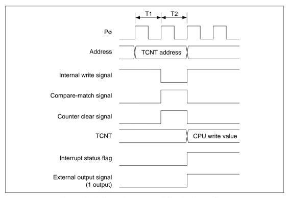
Figure 10.64 Contention between TCNT Write and Clear
