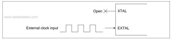
Figure 4.5 External Clock Input Method (Example)
