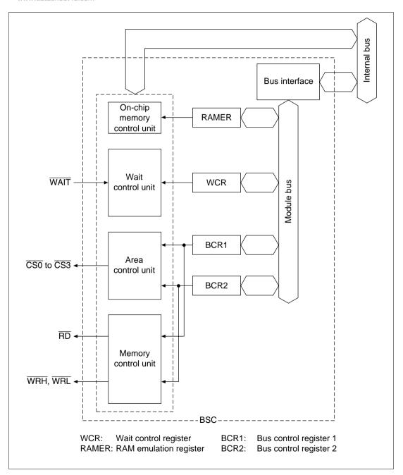
Figure 8.1 BSC Block Diagramwww.DataSheet4U.com
