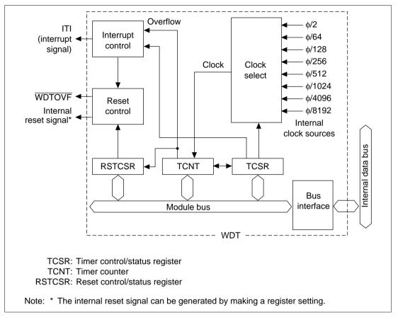
Figure 12.1 WDT Block Diagram
