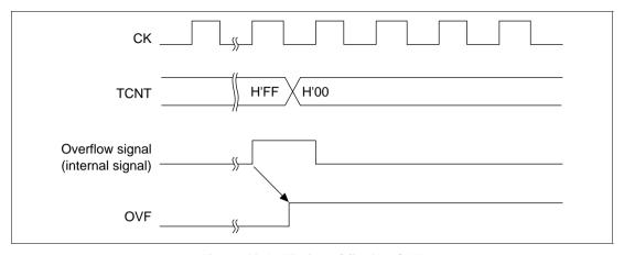
Figure 12.6 Timing of Setting OVF
