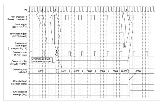
Figure 10.18 Offset One-Shot Pulse Output Function and Output Cutoff Function Operation
