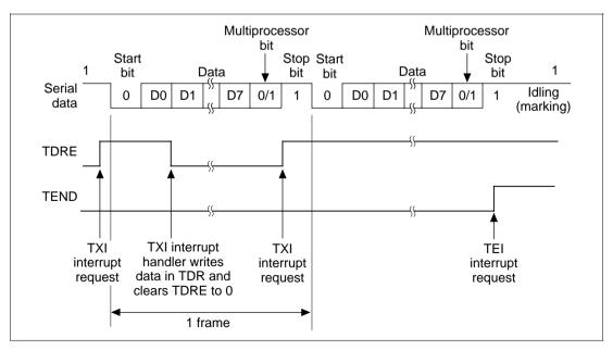
Figure 14.12 SCI Multiprocessor Transmit Operation (Example: 8-Bit Data with Multiprocessor Bit and Operation Bit 4U.com
