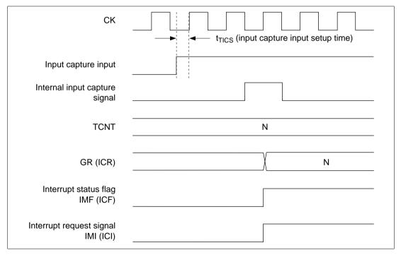
Figure 10.37 IMF (ICF) Setting Timing in Input Capture
