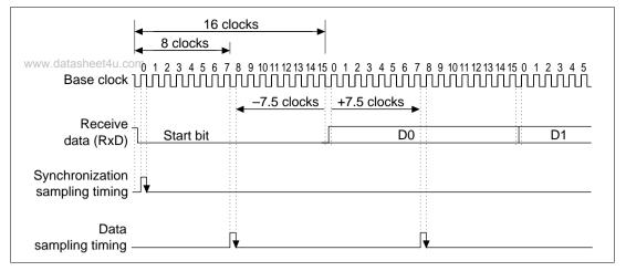
Figure 14.25 Receive Data Sampling Timing in Asynchronous Mode
