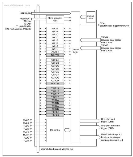
Figure 10.4 Block Diagram of Channel 2
