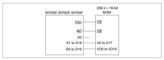
Figure 8.11 Example of 16-Bit Data Bus Width ROM Connection
