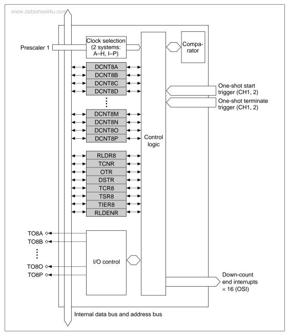
Figure 10.7 Block Diagram of Channel 8
