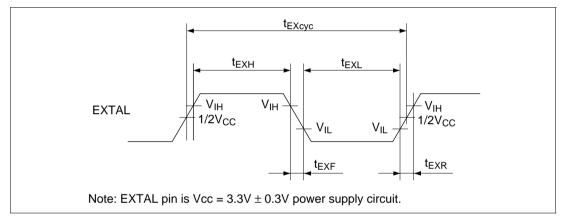
Figure 24.3 EXTAL Clock Input Timing
