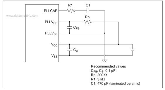
Figure 4.7 Points for Caution in PLL Power Supply Connection
