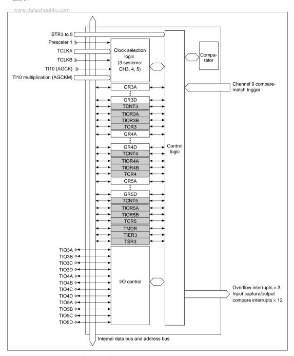
Figure 10.5 Block Diagram of Channels 3 to 5 WWW.DataSheet4U.com
