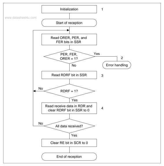
$Figure\ 14.7\quad Sample\ Flowchart\ for\ Receiving\ Serial\ Data\ (1)$
