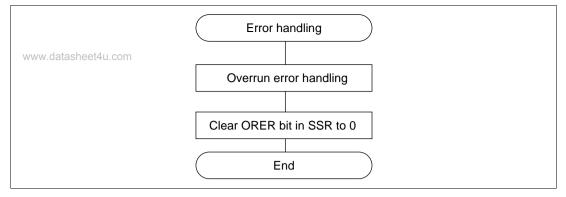
Figure 14.22 Sample Flowchart for Serial Receiving (2)
