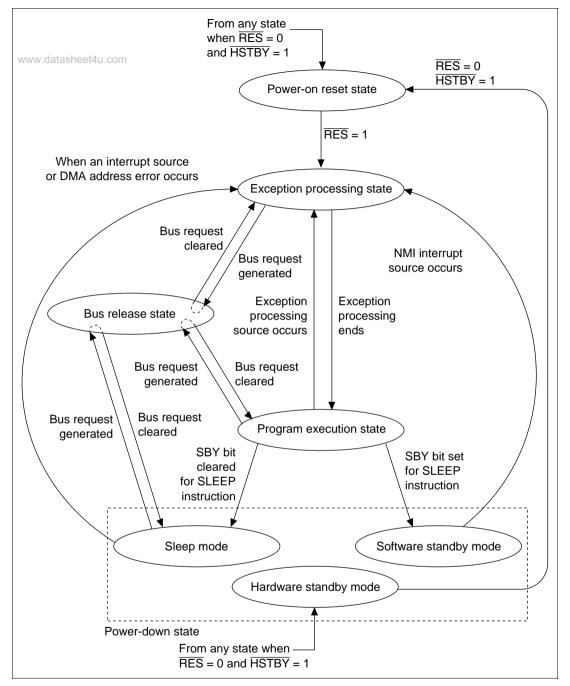
Figure 2.6 Transitions between Processing States
