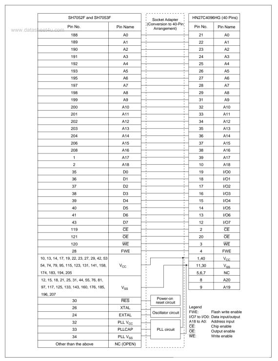
Figure 20.20 Socket Adapter Pin Correspondence Diagramheet 4U.com
