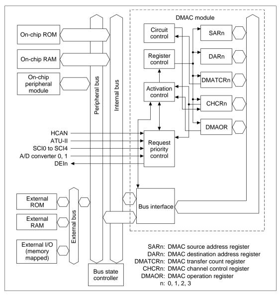
Figure 9.1 DMAC Block Diagraphyw. DataSheet 4U.com
