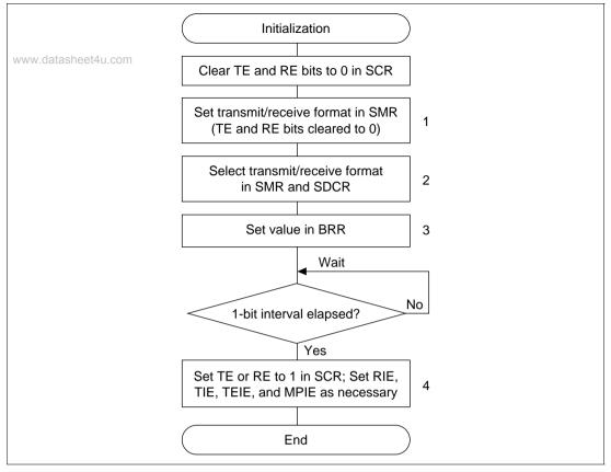
Figure 14.4 Sample Flowchart for SCI Initialization
