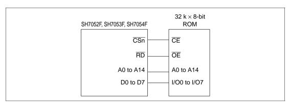
Figure 8.10 Example of 8-Bit Data Bus Width ROM Connection
