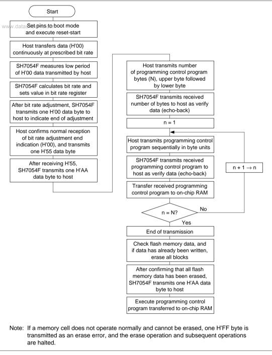
Figure 21.9 Boot Mode Execution Procedure
