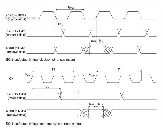
Figure 24.16 SCI Input/Output Timing
