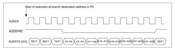
Figure 17.2 Example of Data Output (32-Bit Output)
