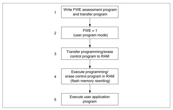
Figure 20.12 User Program Mode Execution Procedure
