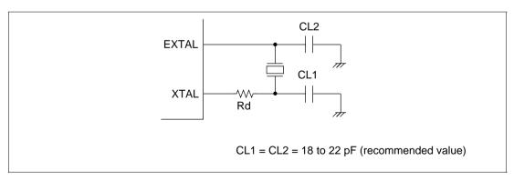
Figure 4.3 Connection of Crystal Oscillator (Example)
