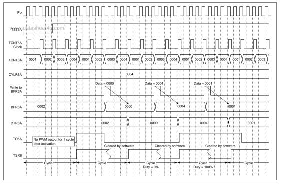
Figure 10.21 PWM Timer Operation
