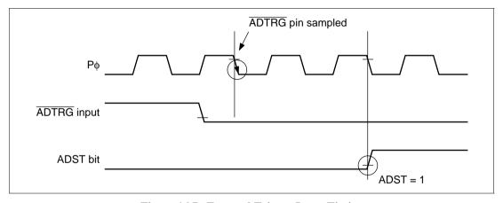
Figure 16.7 External Trigger Input Timing
