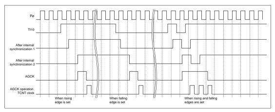
Figure 10.26 Edge Input Operation (Without Noise Cancellation)
