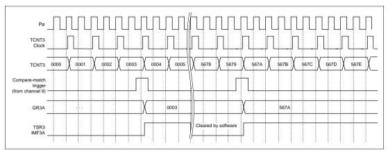
Figure 10.25 Event Cycle Measurement Operation
