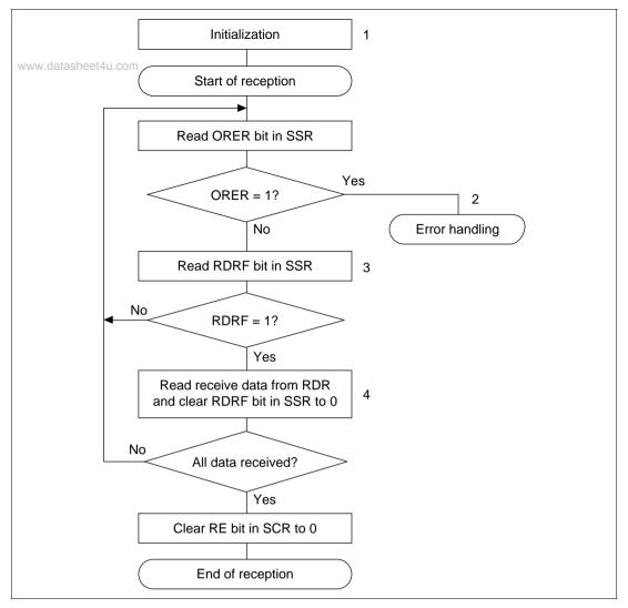
Figure 14.21 Sample Flowchart for Serial Receiving (1)
