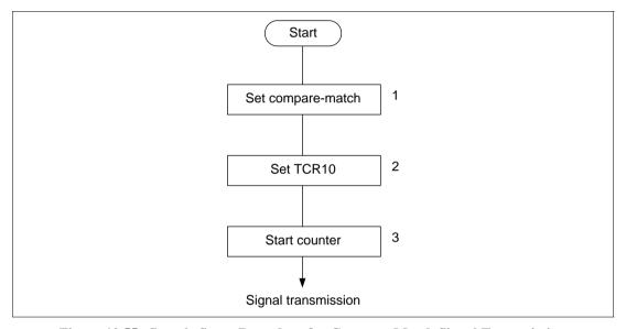
Figure 10.55 Sample Setup Procedure for Compare-Match Signal Transmission
