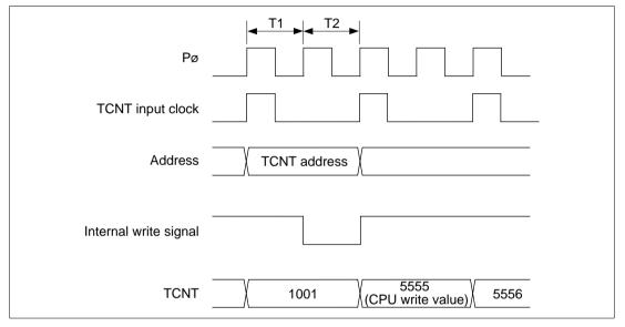
Figure 10.65 Contention between TCNT Write and Increment
