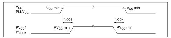
Figure 24.1 Power-On/Off Timing
