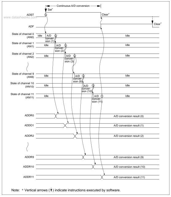
Figure 16.4 Example of A/D Converter Operation (Scan Mode (Single-Cycle Scan), Channels AN0 to AN11 Selected)
