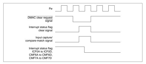
Figure 10.69 Contention between Interrupt Status Flag Clearing by DMAC and Setting by Input Capture/Compare-Match
