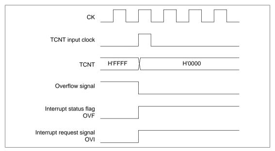
Figure 10.39 OVF Setting Timing in Overflow
