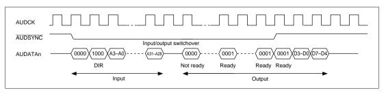
Figure 17.5 Example of Read Operation (Byte Read) a Sheet 4U.com
