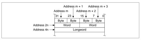
Figure 2.5 Byte, Word, and Longword Alignment
