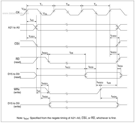
Figure 24.9 Basic Cycle (One Software Wait)
