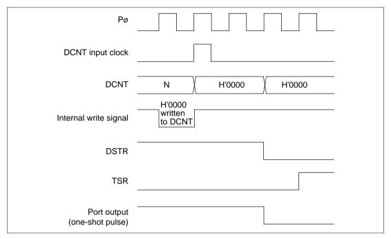
Figure 10.70 Halting of a Down-Counter by the CPU
