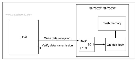
Figure 20.8 System Configuration in Boot Mode
