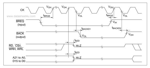
Figure 24.7 Bus Right Release Timing
