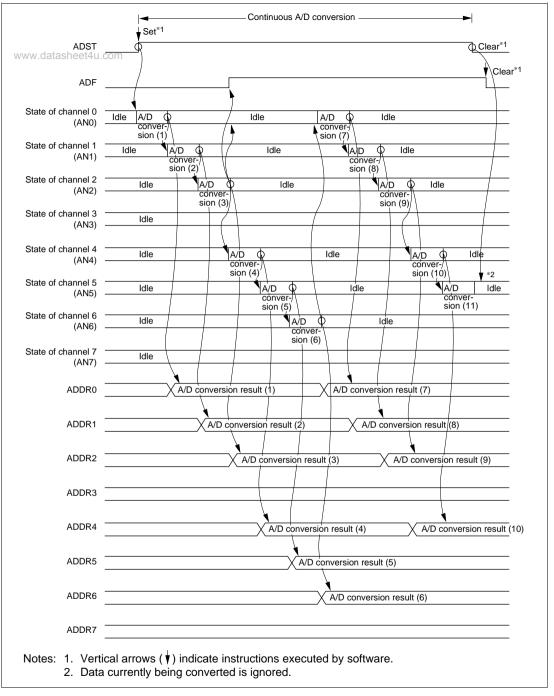
Figure 16.5 Example of A/D Converter Operation (Scan Mode (Continuous Scan), Channels AN0 to AN2 and AN4 to AN6 Selected)
