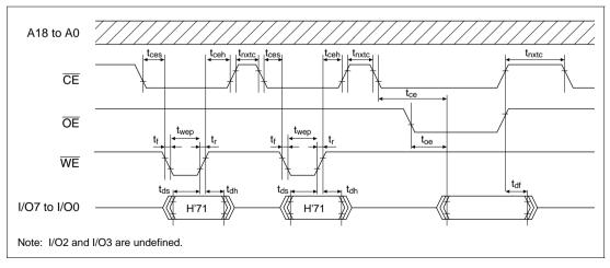
Figure 21.27 Status Read Mode Timing Waveforms
