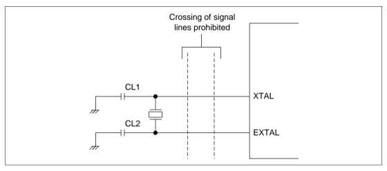
Figure 4.6 Precautions for Oscillator Circuit System Board Design
