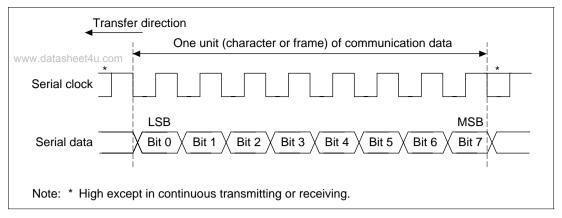
Figure 14.17 Data Format in Synchronous Communication
