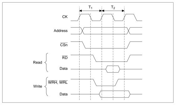
Figure 8.3 Basic Timing of External Space Access
