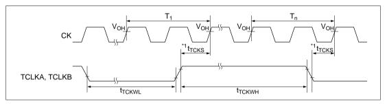
Figure 24.12 ATU Input timing
