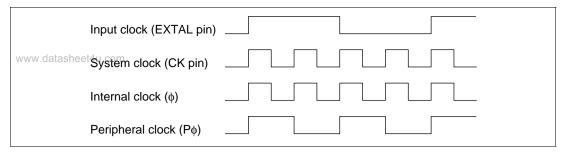
Figure 4.2 Input Clock and System Clock
