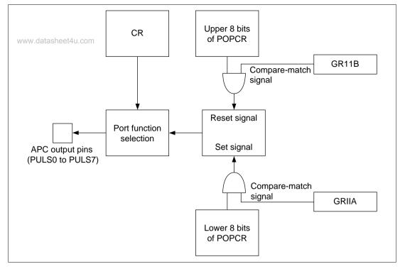
Figure 11.2 Advanced Pulse Controller Output Operation
