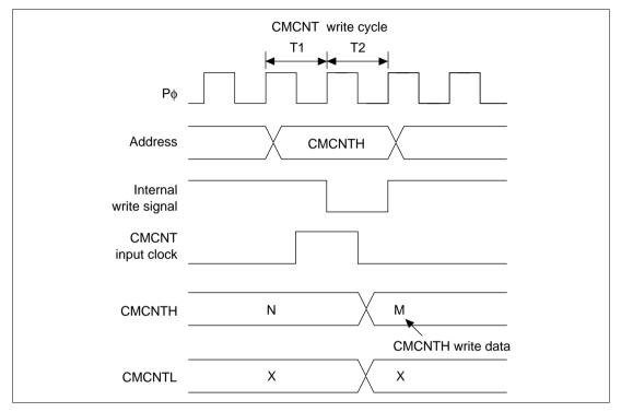
Figure 13.8 CMCNT Byte Write and Increment Contention
