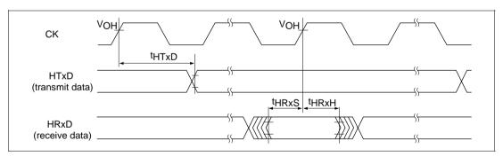
Figure 24.17 HCAN Input/Output timing
