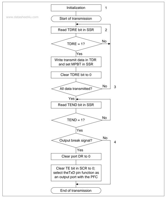
Figure 14.11 Sample Flowchart for Transmitting Multiprocessor Serial Data
