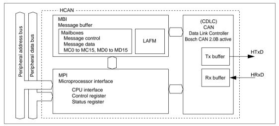
Figure 15.1 HCAN Block Diagram
