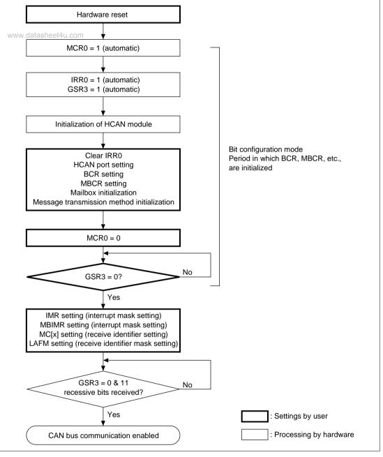
Figure 15.5 Hardware Reset Flowchart
