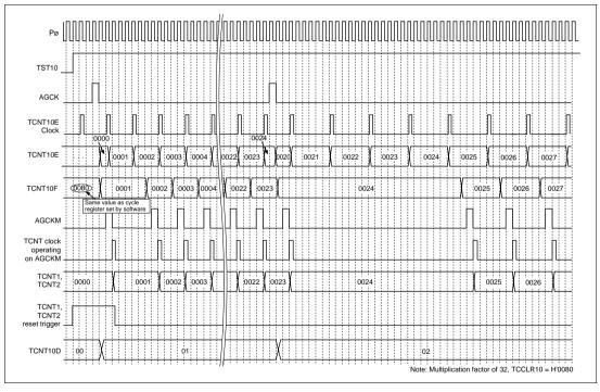
Figure 10.34 TCNT10F Operation (At Startup)
