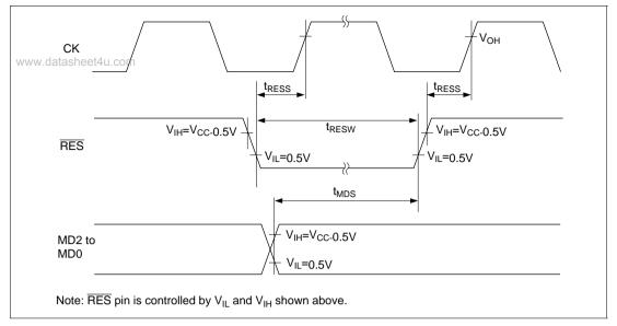
Figure 24.5 Reset Input Timing
