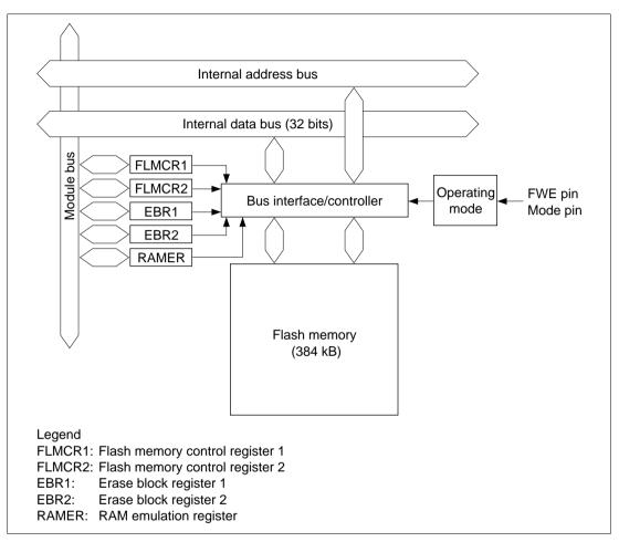
Figure 21.1 Block Diagram of Flash Memory
