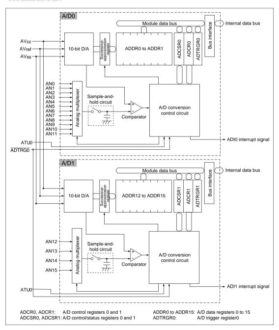
Figure 16.1 A/D Converter Block Diagram WWW.DataSheet4U.com
