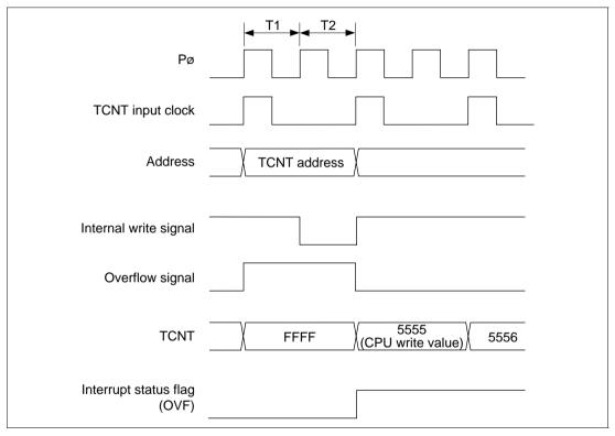
Figure 10.66 Contention between TCNT Write and Overflow
