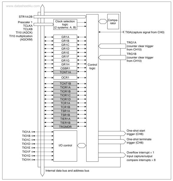
Figure 10.3 Block Diagram of Channel 1
