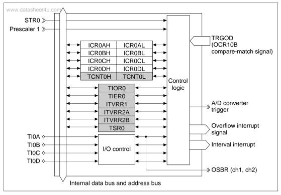
Figure 10.2 Block Diagram of Channel 0
