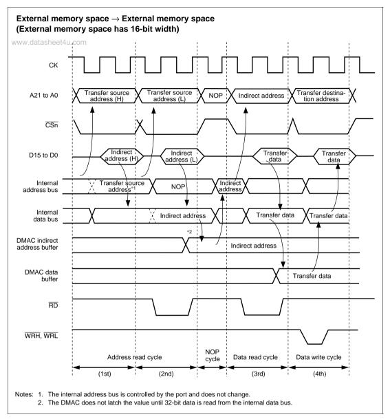
Figure 9.6 Dual Address Mode and Indirect Address Transfer Timing Example 1
