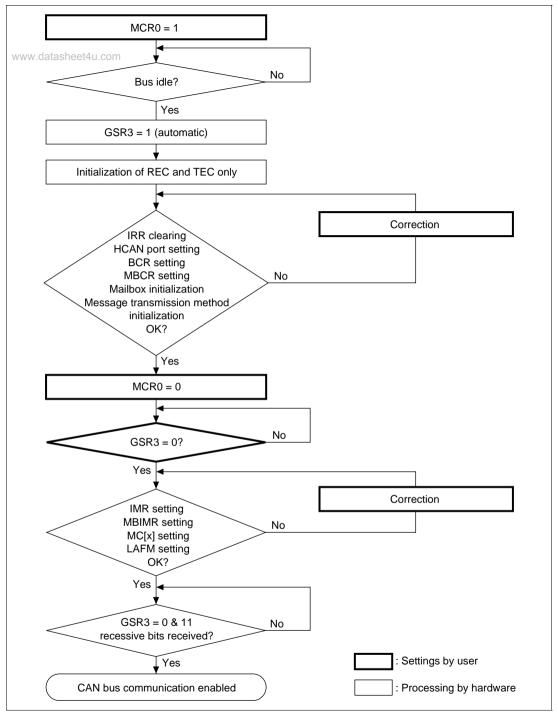
Figure 15.6 Software Reset Flowchart
