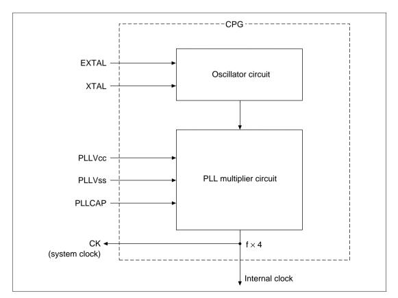
Figure 4.1 Block Diagram of Clock Pulse Generate a Sheet 4U.com
