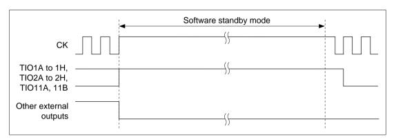
Figure 10.74 External Output Value Transition Points in Relation to Software Standby Mode
