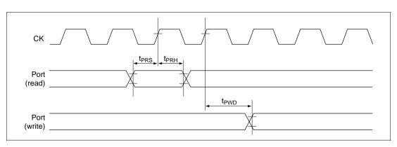
Figure 24.13 I/O Port Input/Output timing
