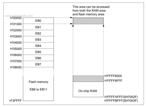
Figure 20.18 Example of RAM Overlap Operation
