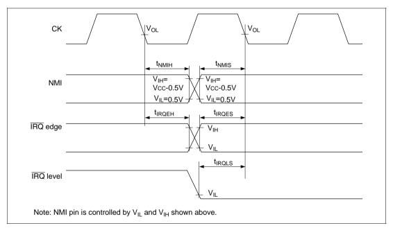
Figure 24.6 Interrupt Signal Input Timing
