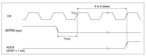
Figure 24.18 External Trigger Input Timing
