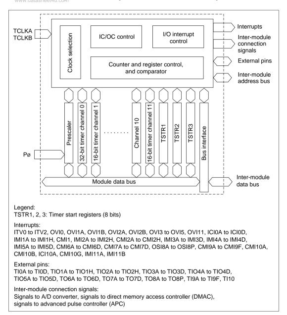
Figure 10.1 Overall Block Diagram of ATU-II
