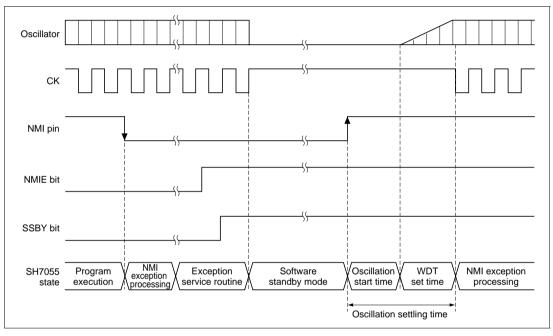
Figure 23.3 Software Standby Mode NMI Timing (Application Example)
