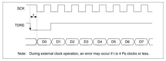
Figure 14.26 Example of Synchronous Transmission with DMAC
