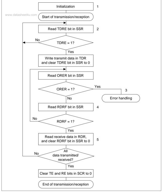
Figure 14.24 Sample Flowchart for Serial Transmission and Reception
