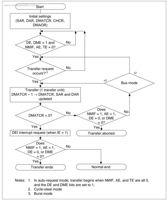
Figure 9.2 DMAC Transfer Flowchart
