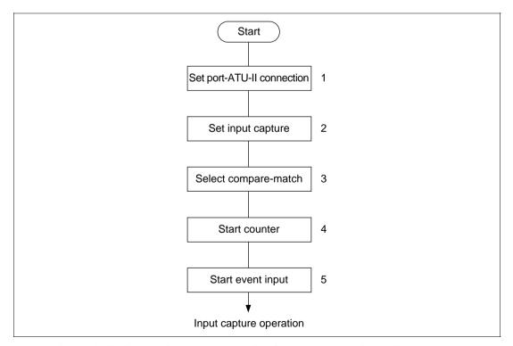
Figure 10.62 Sample Setup Procedure for Compare-Match Signal Transmission
