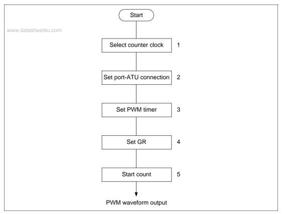
Figure 10.59 Sample Setup Procedure for PWM Timer Operation (Channels 3 to 5)
