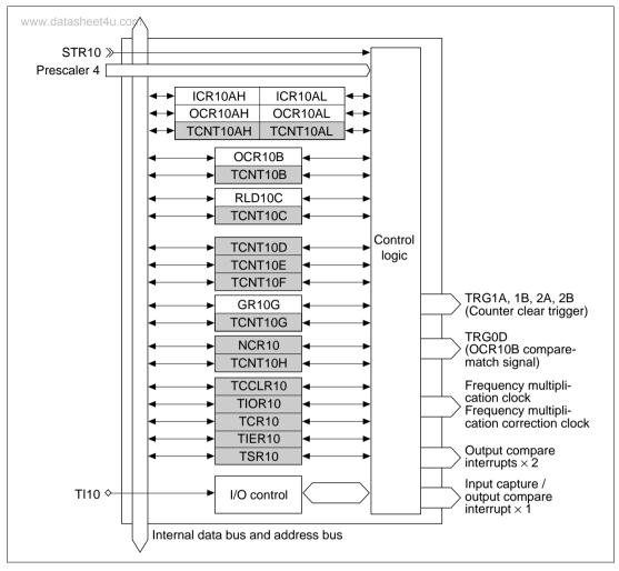
Figure 10.9 Block Diagram of Channel 10
