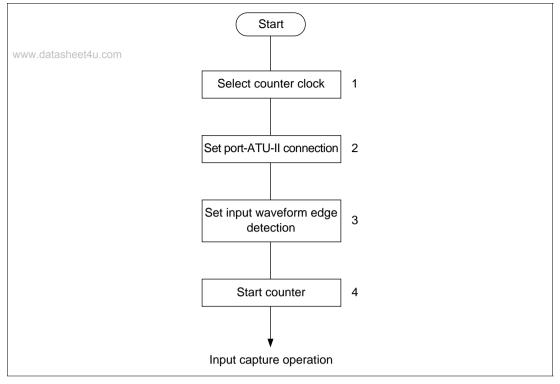
Figure 10.53 Sample Setup Procedure for Input Capture
