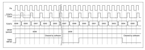
Figure 10.14 Example of Cyclic Counter Operation
