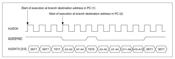
Figure 17.3 Example of Output in Case of Successive Branches
