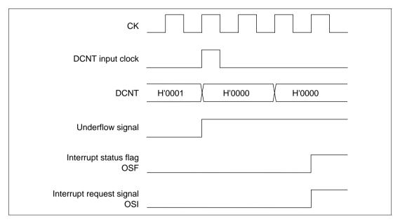
Figure 10.40 OSF Setting Timing in Underflow
