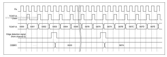
Figure 10.20 Twin-Capture Operation
