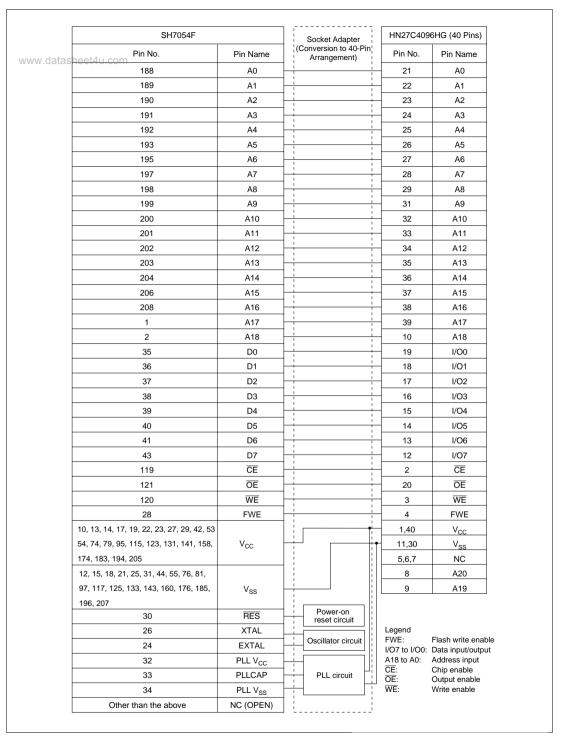
Figure 21.20 Socket Adapter Pin Correspondence Diagramheet 4U.com
