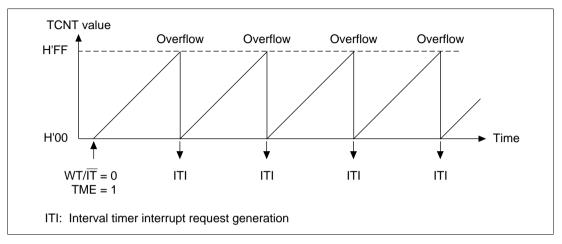
Figure 12.5 Operation in Interval Timer Mode
