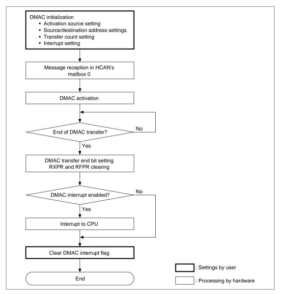
Figure 15.13 DMAC Transfer Flowchart
