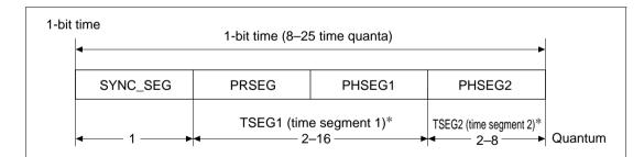
SYNC\_SEG: Segment for establishing synchronization of nodes on the CAN bus. (Normal
