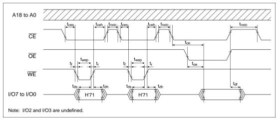
Figure 20.27 Status Read Mode Timing Waveforms
