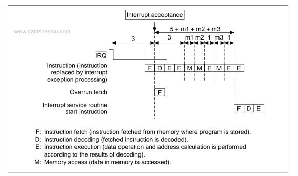
Figure 6.4 Example of Pipeline Operation when an IRQ Interrupt is Accepted
