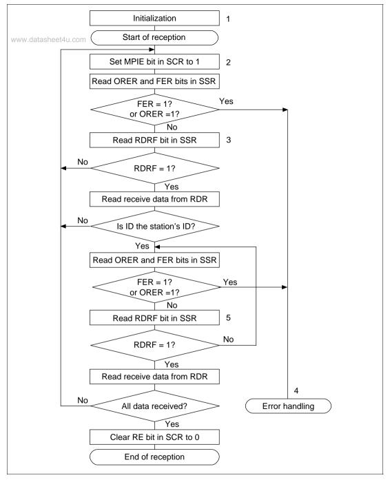
Figure 14.13 Sample Flowchart for Receiving Multiprocessor Serial Data (1)
