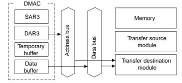
The DAR3 value is taken as the address, and the value in the data buffer is written to the transfer destination module.
