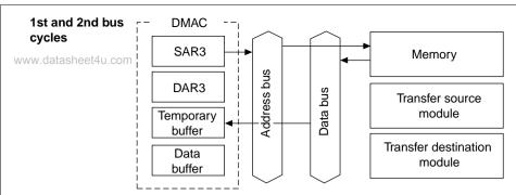
The SAR3 value is taken as the address, memory data is read, and the value is stored in the temporary buffer. Since the value read at this time is used as the address, it must be 32 bits. If the data bus is 16 bits wide when the external memory space is accessed, two bus cycles are necessary.
