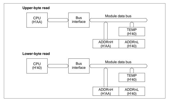
Figure 16.2 A/D Data Register Access Operation (Reading H'AA40)
