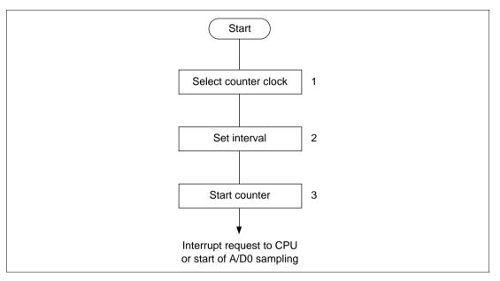
Figure 10.58 Sample Setup Procedure for Interval Timer Operation
