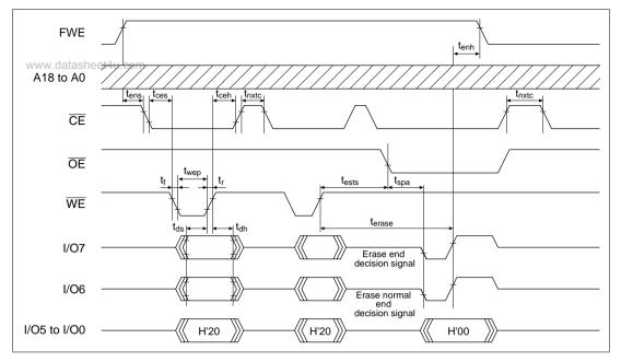
Figure 21.26 Auto-Erase Mode Timing Waveforms
