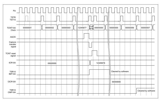
Figure 10.28 TCNT10A Capture Operation and Compare-Match Operation
