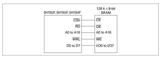
Figure 8.12 Example of 8-Bit Data Bus Width SRAM Connection www.DataSheet4U.com
