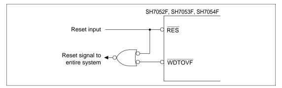
Figure 12.9 Example of System Reset Circuit Using WDTOVF Signal
