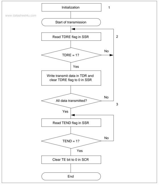
Figure 14.19 Sample Flowchart for Serial Transmitting
