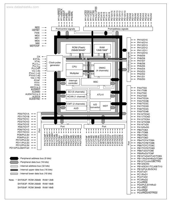
Figure 1.1 Block Diagram
