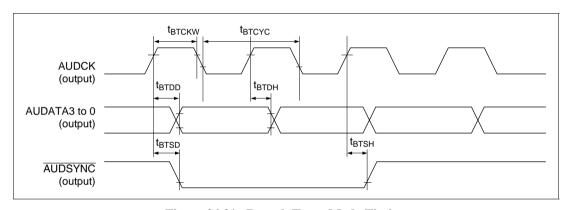
Figure 24.21 Branch Trace Mode Timing
