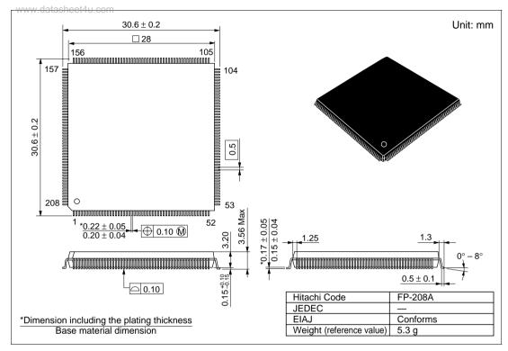
Figure D.1 Package Dimensions (FP-208A)
