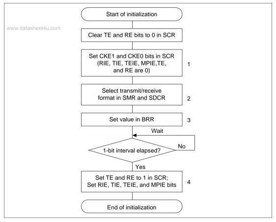
Figure 14.18 Sample Flowchart for SCI Initialization
