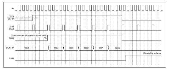
Figure 10.17 One-Shot Pulse Output Operation
