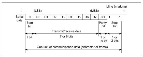
Figure 14.2 Data Format in Asynchronous Communication (Example: 8-bit Data with Parity and Two Stop Bits)
