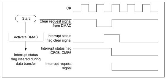
Figure 10.43 Procedure and Timing for Clearing by DMAC
