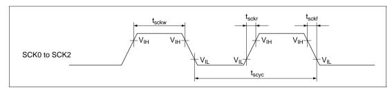
Figure 24.15 SCI Input/Output Timing
