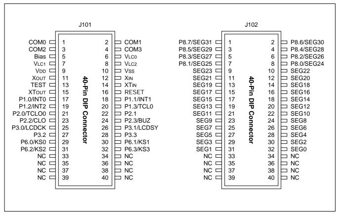
Figure 17-3. 40-Pin Connectors for TB7574
