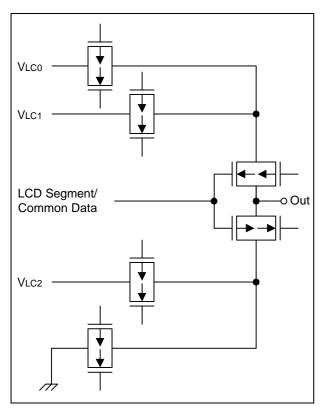
Figure 1-8. Pin Circuit Type H (SEG/COM)
