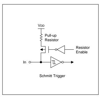
Figure 1-5. Pin Circuit Type A-4 (P1)
