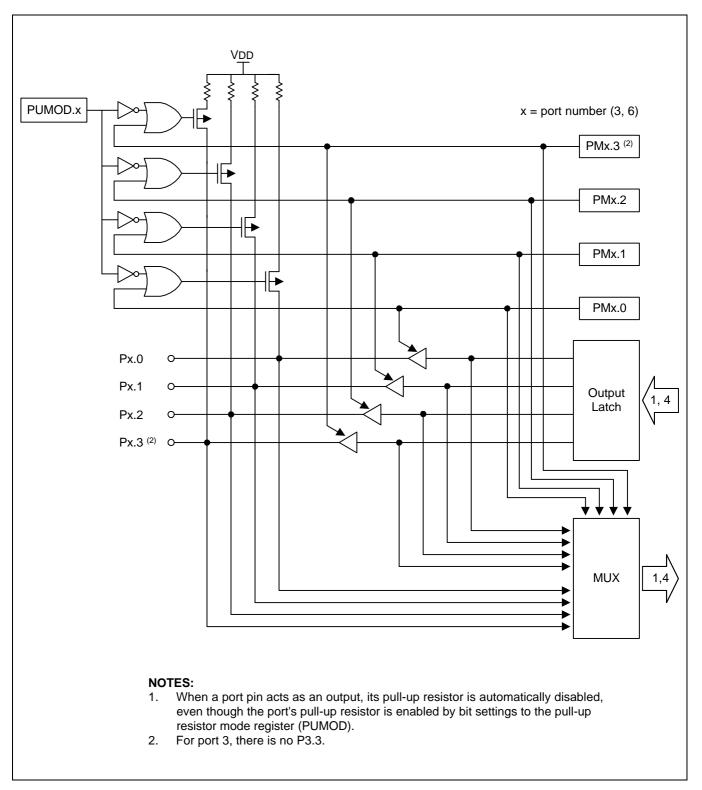
Figure 10-3. Ports 3 and 6 Circuit Diagram
