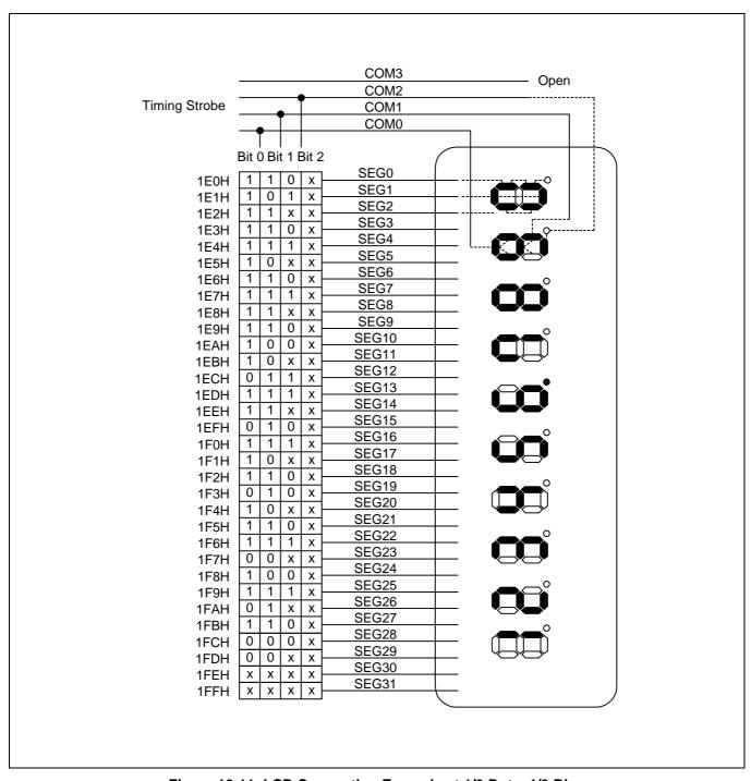
Figure 12-11. LCD Connection Example at 1/3 Duty, 1/3 Bias
