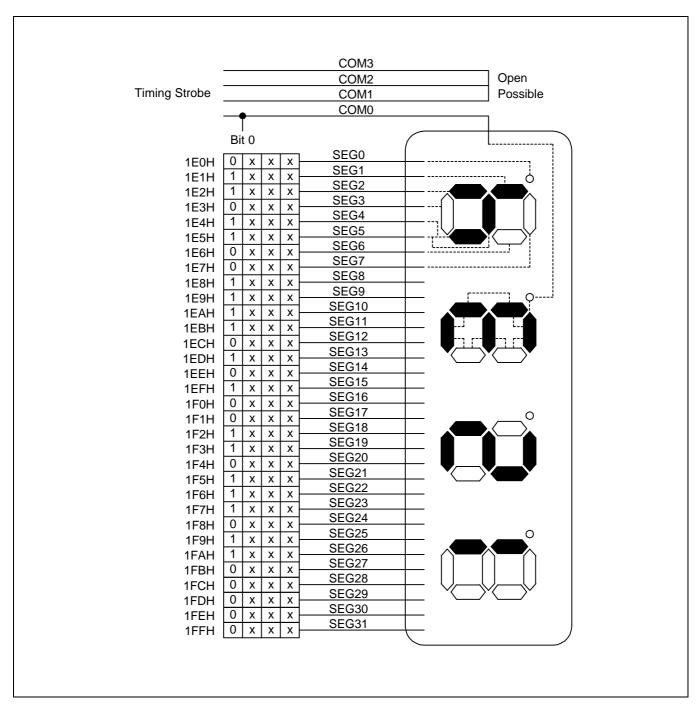
Figure 12-6. LCD Connection Example in Static Mode
