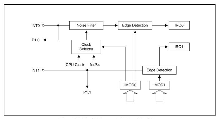
Figure 7-5. Circuit Diagram for INT0 and INT1 Pins
