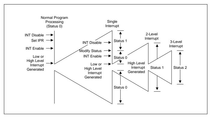
Figure 7-4. Multi-Level Interrupt Handling
