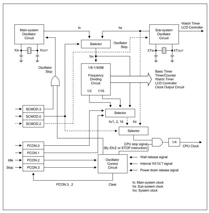
Figure 6-1. Clock Circuit Diagram
