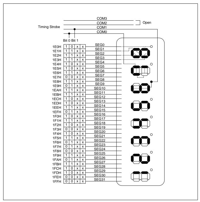
Figure 12-8. LCD Connection Example at 1/2 Duty, 1/2 Bias
