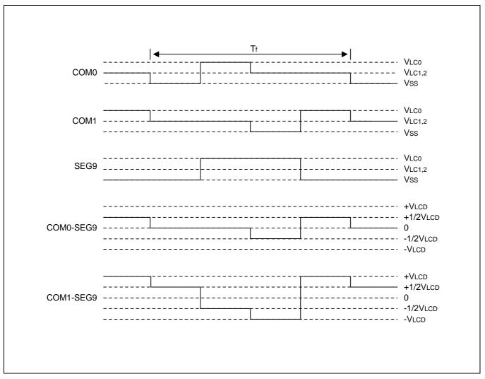
Figure 12-7. LCD Signal Waveforms at 1/2 Duty, 1/2 Bias
