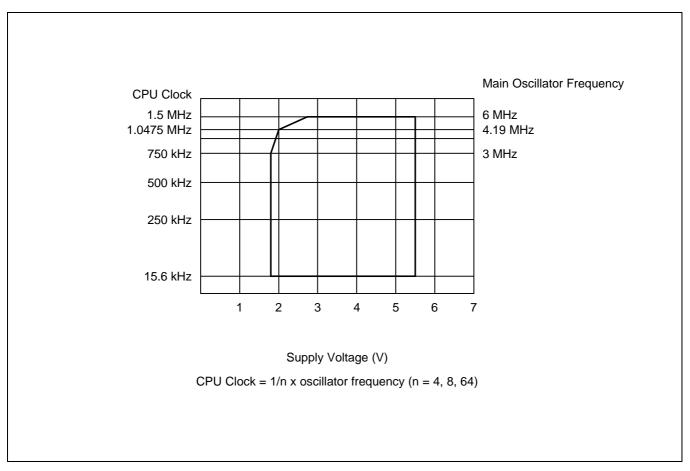
Figure 14-1. Standard Operating Voltage Range
