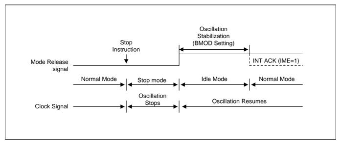
Figure 8-4. Timing When Main Stop or Main/Sub Stop Mode is Release by an Interrupt
