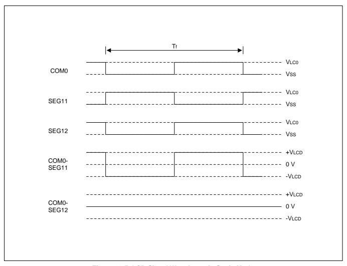
Figure 12-5. LCD Signal Waveforms in Static Mode
