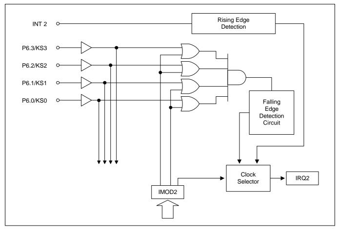
Figure 7-6. Circuit Diagram for INT2 and KS0-KS3 Pins
