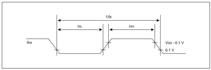
Figure 14-5. Clock Timing Measurement at X<sub>IN</sub>
