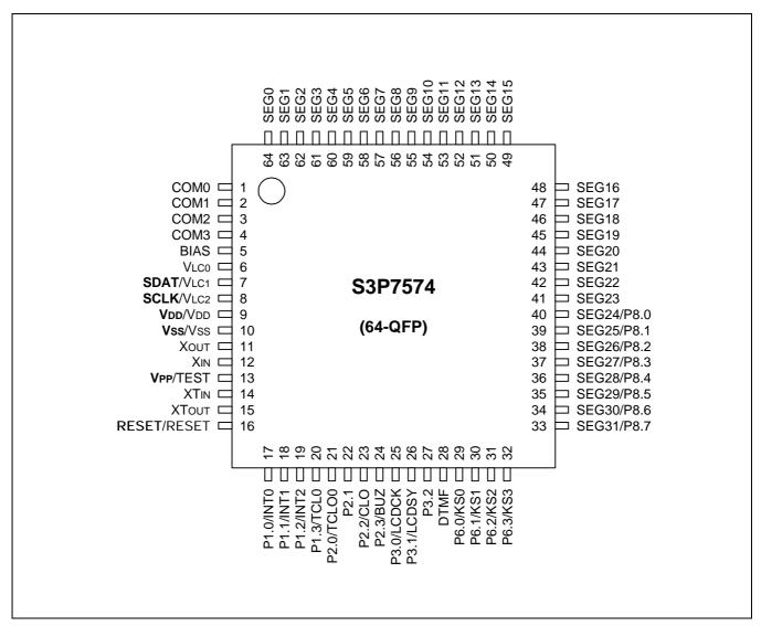
Figure 16-2. S3P7574 Pin Assignments (64-QFP)
