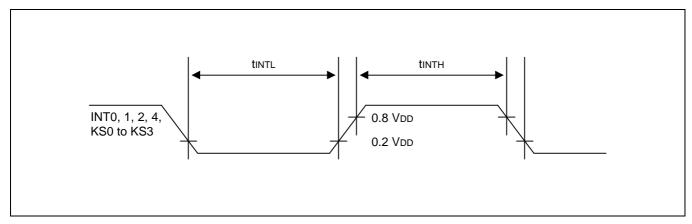
Figure 14-9. Input Timing for External Interrupts and Quasi-Interrupts
