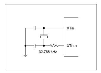
Figure 6-5. Crystal/Ceramic Oscillator
