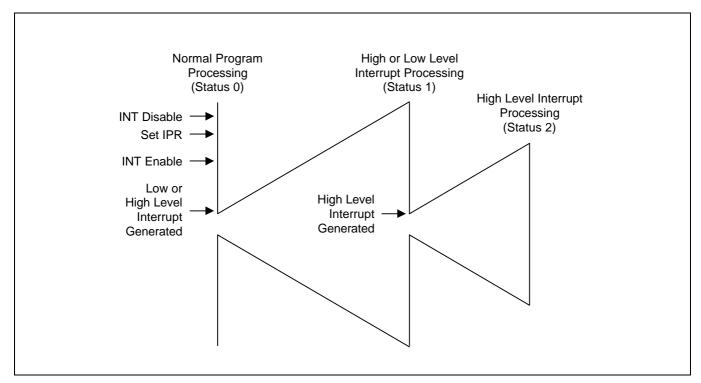
Figure 7-3. Two-Level Interrupt Handling
