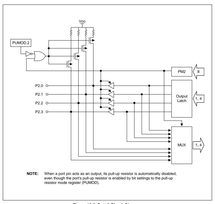
Figure 10-2. Port 2 Circuit Diagram
