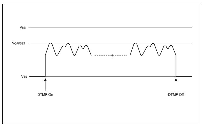
Figure 13-1. DTMF Output Waveform
