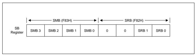
Figure 3-2. SMB and SRB Values in the SB Register
