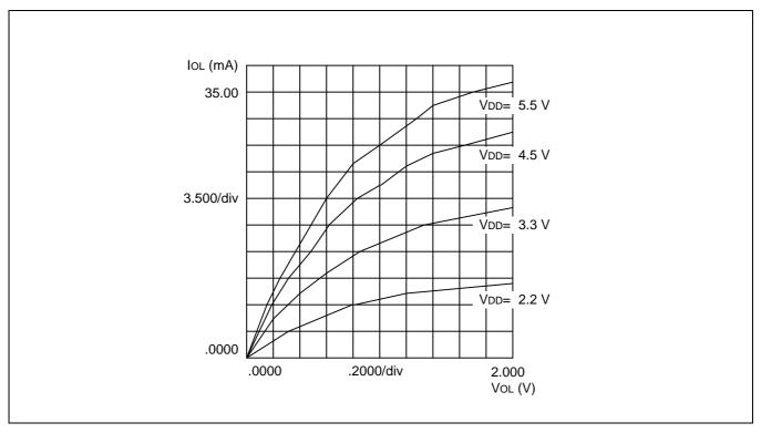
Figure 16-4. Port 2  $I_{OL}$  vs  $V_{OL}$  Curve
