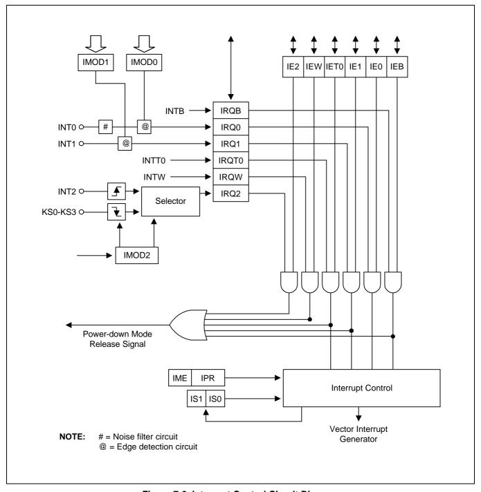
Figure 7-2. Interrupt Control Circuit Diagram
