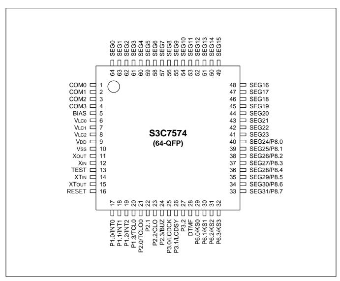
Figure 1-3. S3C7574 64-QFP Pin Assignment
