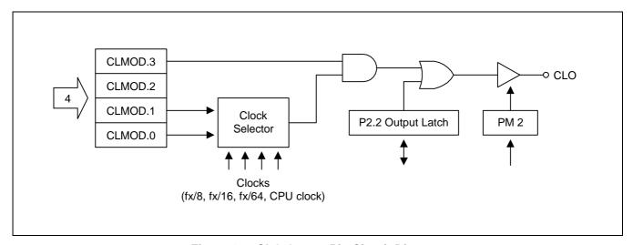
Figure 6-7. CLO Output Pin Circuit Diagram
