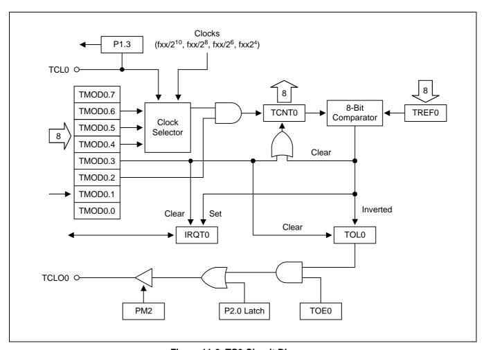
Figure 11-2. TC0 Circuit Diagram
