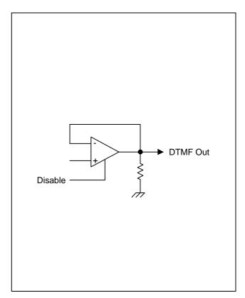
Figure 1-11. Pin Circuit Type G-6 (DTMF)
