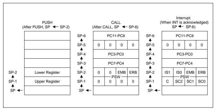
Figure 2-7. Push-Type Stack Operations
