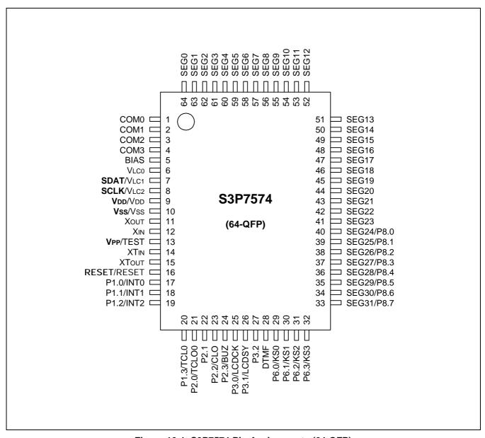
Figure 16-1. S3P7574 Pin Assignments (64-QFP)
