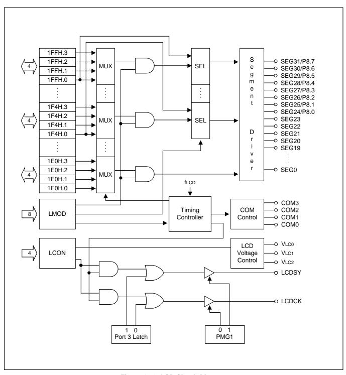
Figure 12-2. LCD Circuit Diagram
