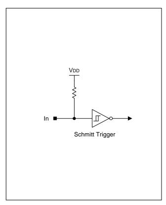
Figure 1-10. Pin Circuit Type B (RESET)
