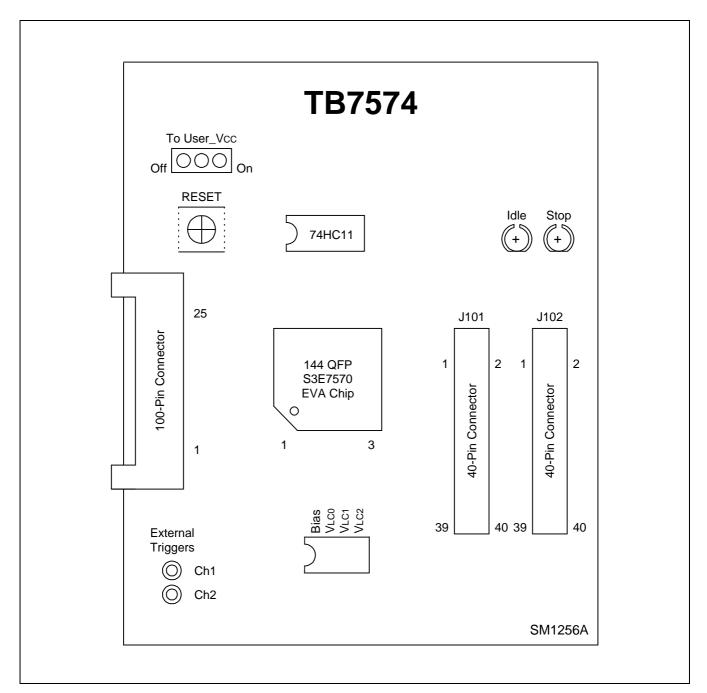
Figure 17-2. TB7574 Target Board Configuration
