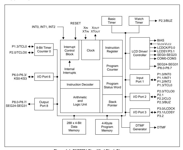
Figure 1-1. S3C7574 Simplified Block Diagram
