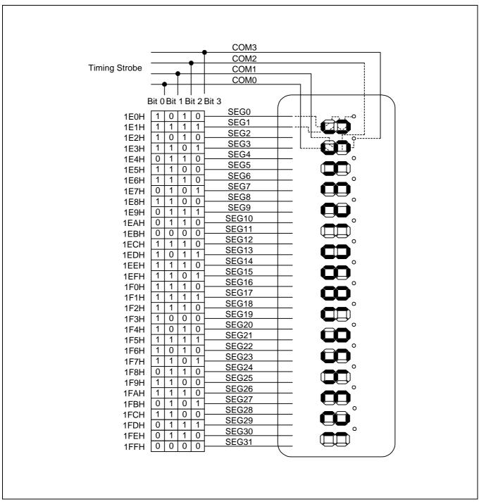
Figure 12-13. LCD Connection Example at 1/4 Duty, 1/3 Bias
