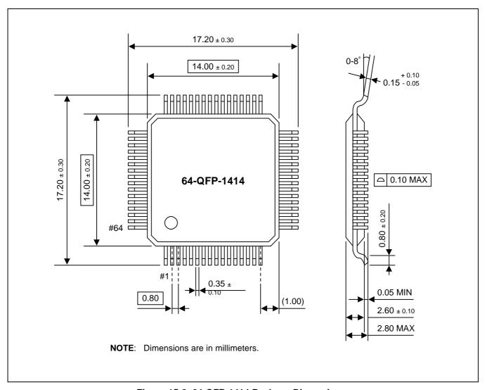
Figure 15-2. 64-QFP-1414 Package Dimensions.
