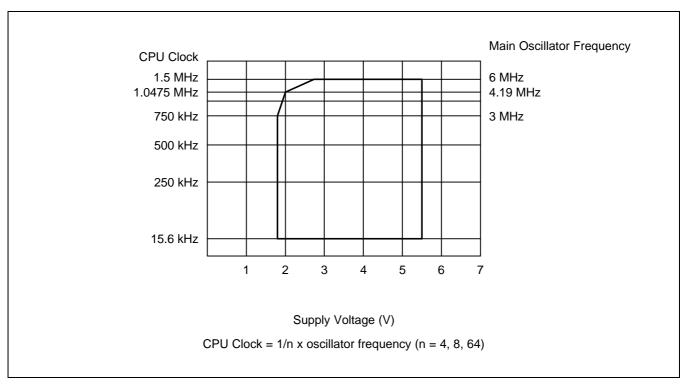
Figure 16-3. Standard Operating Voltage Range
