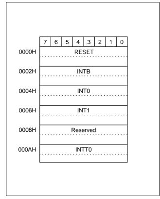
Figure 2-2. Vector Address Structure
