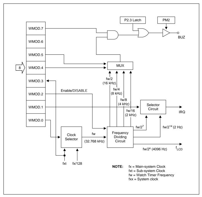
Figure 11-4. Watch Timer Circuit Diagram
