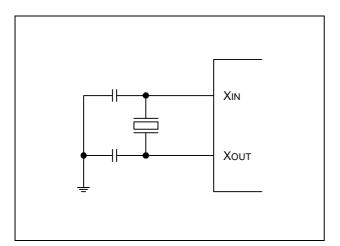
Figure 6-2. Crystal/Ceramic Oscillator
