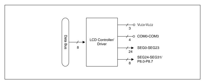
Figure 12-1. LCD Function Diagram
