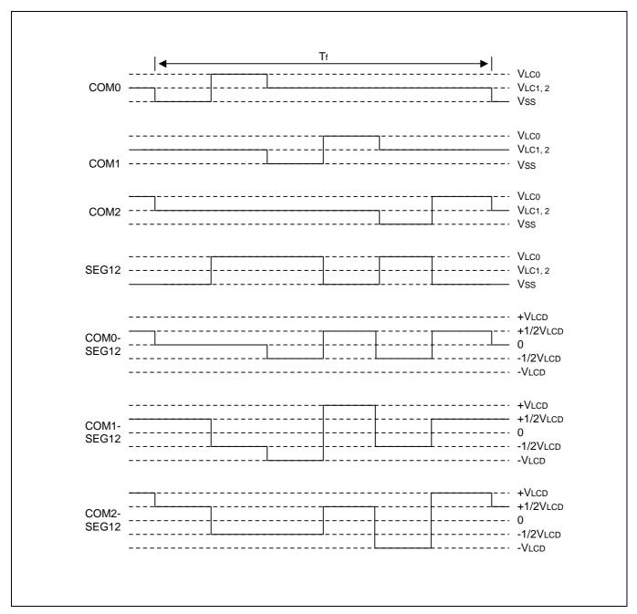
Figure 12-9. LCD Signal Waveforms at 1/3 Duty, 1/2 Bias
