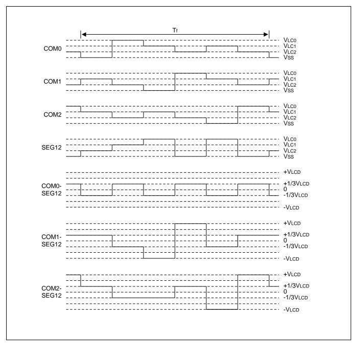
Figure 12-10. LCD Signal Waveforms at 1/3 Duty, 1/3 Bias
