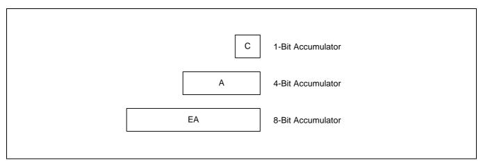
Figure 2-6. 1-Bit, 4-Bit, and 8-Bit Accumulator
