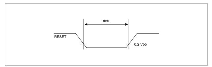
Figure 14-8. Input Timing for RESET Signal
