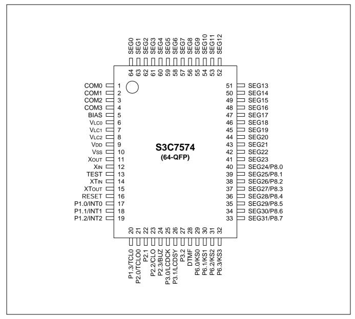
Figure 1-2. S3C7574 64-QFP Pin Assignment
