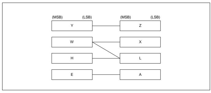
Figure 2-5. Register Pair Configuration
