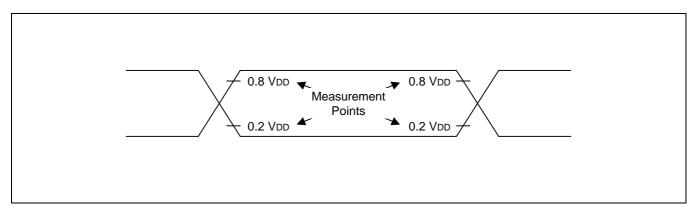
Figure 14-4. A.C. Timing Measurement Points (Except for X<sub>IN</sub> and XT<sub>IN</sub>)
