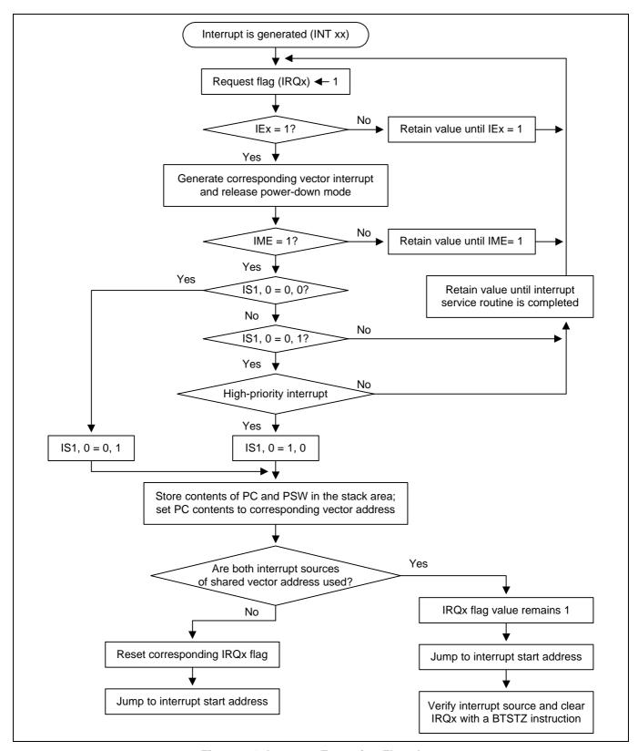
Figure 7-1. Interrupt Execution Flowchart
