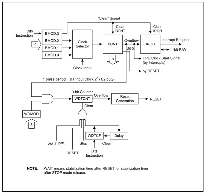
Figure 11-1. Basic Timer Circuit Diagram
