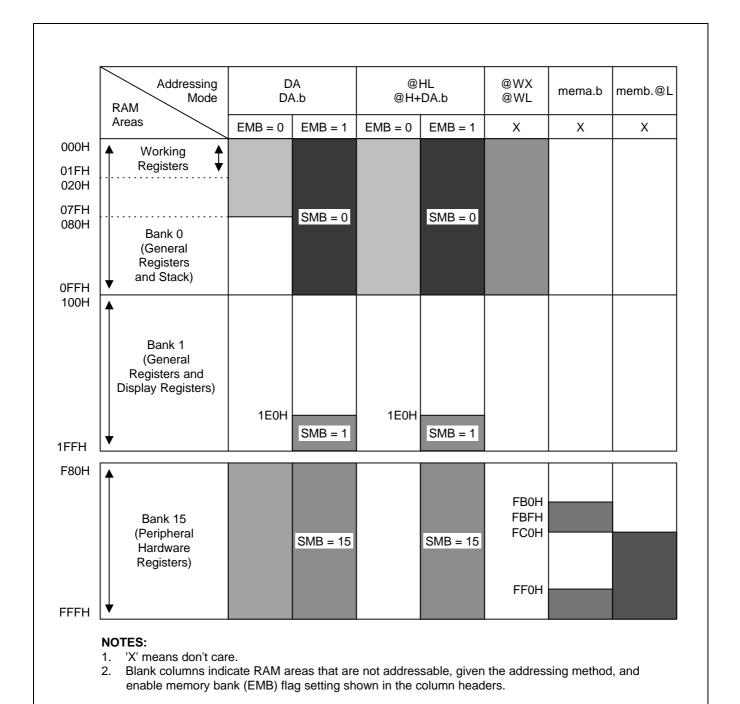
Figure 3-1. RAM Address Structure
