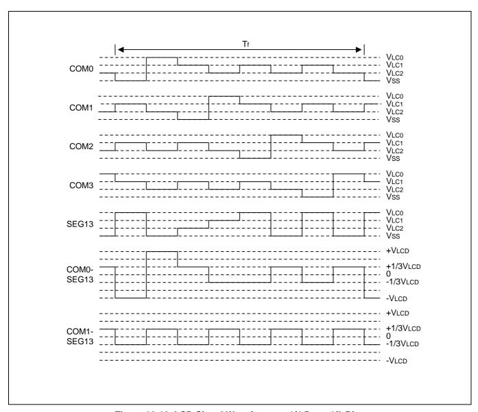
Figure 12-12. LCD Signal Waveforms at 1/4 Duty, 1/3 Bias
