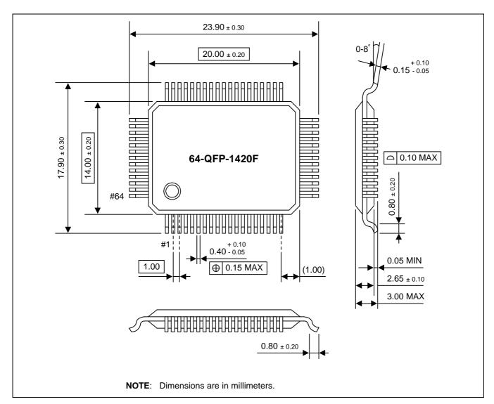
Figure 15-1. 64-QFP-1420F Package Dimensions
