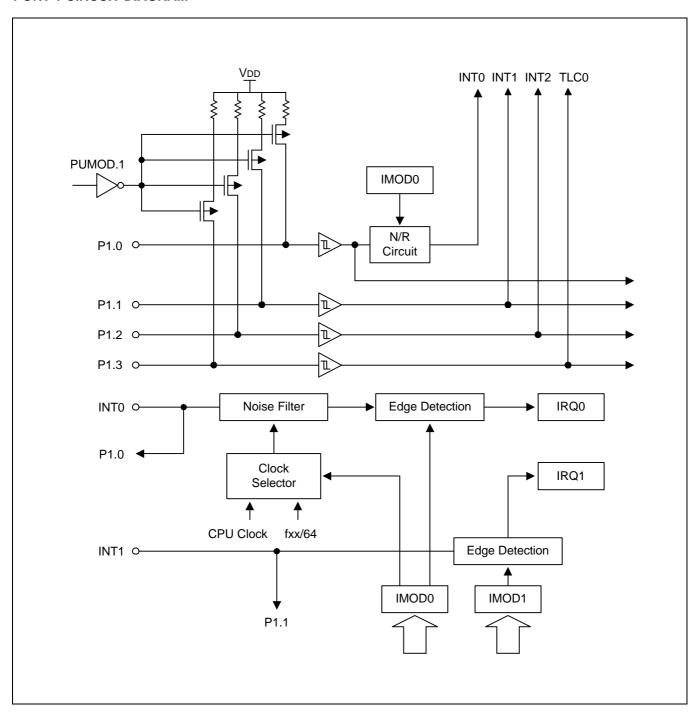
Figure 10-1. Input Port 1 Circuit Diagram
