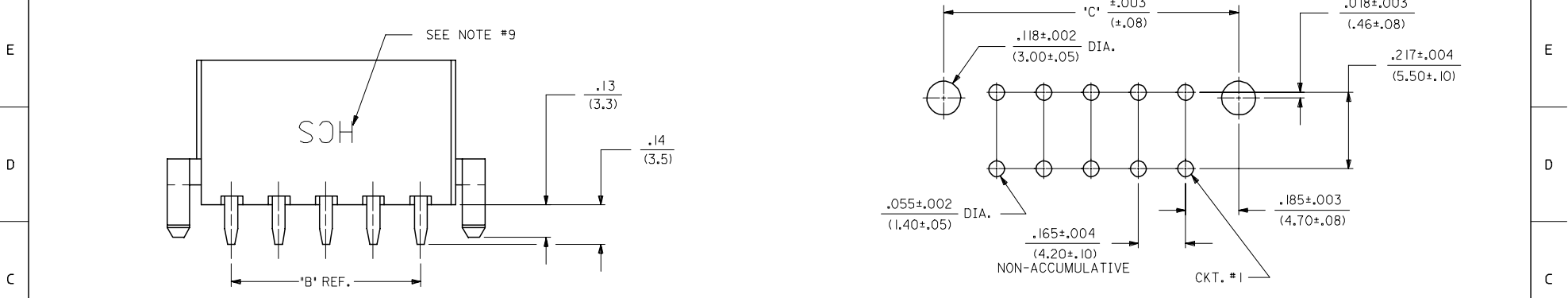
RECOMMENDED HOLE LAYOUT FOR .070/(1.78) MAX. THICK P. C. BOARD VIEWED FROM COMPONENT SIDE
