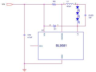
A value of 1uF will reduce the supply ripple current by a factor three (approx.). Proportionally lower ripple can be achieved with higher capacitor values. Note that the capacitor will not affect operating frequency or efficiency, but it will increase start-up delay and reduce the frequency of dimming, by reducing the rate of rise of LED voltage. By adding this capacitor the current waveform through the LED(s) changes from a triangular ramp to a more sinusoidal version without altering the
