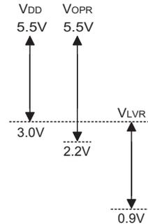
Note:  $V_{\text{OPR}}$  is the voltage range for proper chip operation at 4MHz system clock.
