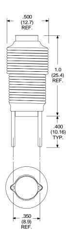
Height dimensions are without solder joint or coatings
