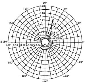
$\begin{array}{l} S_{22e} \\ V_{CE} = 10V \\ I_{C} = 20 mA \\ T_{a} = 25 ^{\circ}C \\ (Unit: \Omega) \end{array}$
