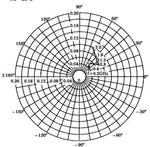
$\begin{array}{l} S_{22e} \\ V_{CE} = 10V \\ I_{C} = 5 \text{mA} \\ T_{a} = 25 ^{\circ}\text{C} \\ \text{(Unit : } \Omega\text{)} \end{array}$
