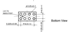
Fig3. VCSP50L1 Package (Unit; mm)
