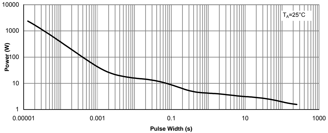
Figure 11: Single Pulse Power Rating Junction-to-Ambient (Note F)
