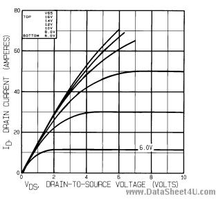
Figure 17. – Typical Output Characteristics Post-Radiation 1 Mega Rads (Si)
