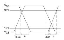
Figure 28b. - Switching Time Waveforms
