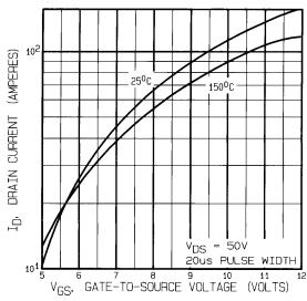
www.DataSheet4U.com Figure 20. - Typical Transfer Characteristics
