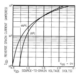
Figure 24. – Typical Source-Drain Diode Forward Voltage
