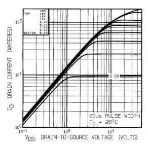
Figure 18. - Typical Output Characteristics, TC = 25°C
