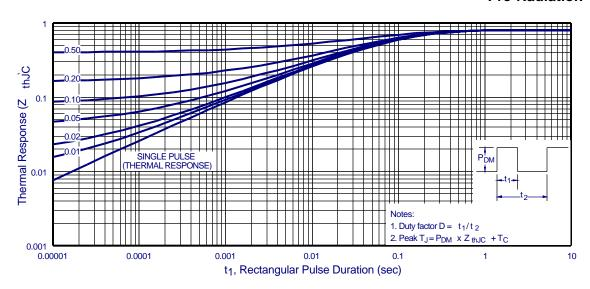
Figure 26. - Maximum Effective Transient Thermal Impedance, Junction-to-Case Vs. Pulse Duration
