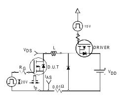
Figure 29a. - Unclamped Inductive Test Curcuit
