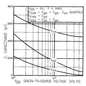
Figure 22. – Typical Capacitance Vs. Drain-to-Source Voltage
