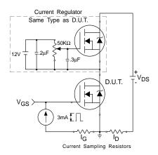
Figure 31b. - Gate Charge Test Circuit
