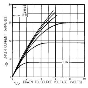
Figure 16. – Typical Output Characteristics Post-Radiation 300K Rads (Si)
