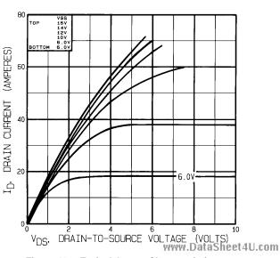
Figure 13. – Typical Output Characteristics Post-Radiation 1 Mega Rads (Si)
