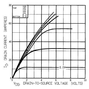
Figure 10. – Typical Output Characteristics
