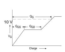
Figure 31a. – Basic Gate Charge Waveform
