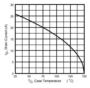
Figure 27. - Maximum Drain Current Vs. Case Temperature
