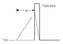
Figure 29b. - Unclamped Inductive Waveforms
