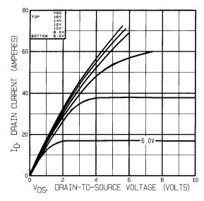
Figure 12. – Typical Output Characteristics Post-Radiation 300K Rads (Si)
