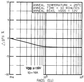
Figure 3. – Typical Response of Transconductance Vs.
