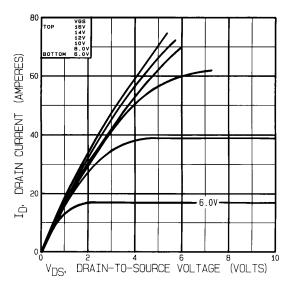
Figure 15. – Typical Output Characteristics Post-Radiation 100K Rads (Si)
