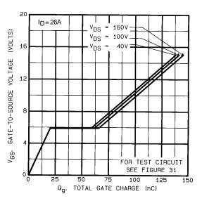
Figure 23. – Typical Gate Charge Vs. Gate-to-Source Voltage
