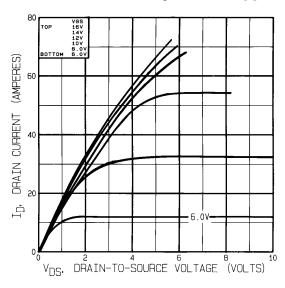
Figure 14. – Typical Output Characteristics Pre-Radiation
