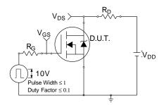
Figure 28a. - Switching Time Test Circuit
