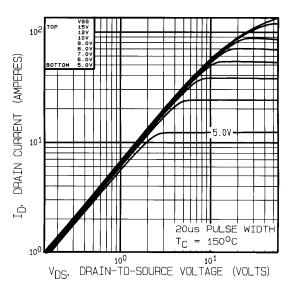
Figure 19. - Typical Output Characteristics, Tc = 150°C
