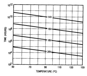
Figure 32 - Typical Time to Accumulated 1% Failure
