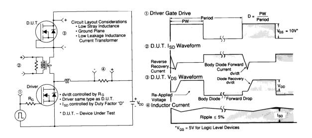
Figure 30. - Peak Diode Recovery dv/dt Test Circuit
