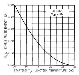
Figure 29c. – Maximum Avalanche Energy Vs. Starting Junction Temperature
