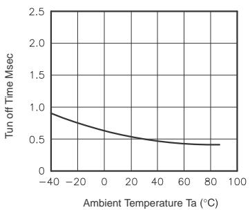
**Fig.5** LED operate vs. ambient temperature
