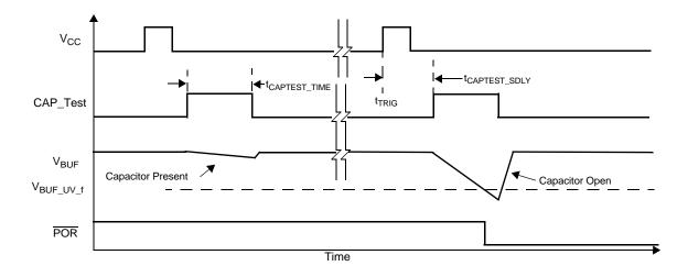
Figure 11. V<sub>BUF</sub> Capacitor Monitor - Synchronous Mode
