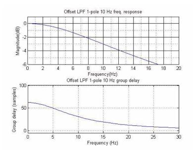
Figure 20. 10Hz Offset Cancellation Low Pass Filter Characteristics
