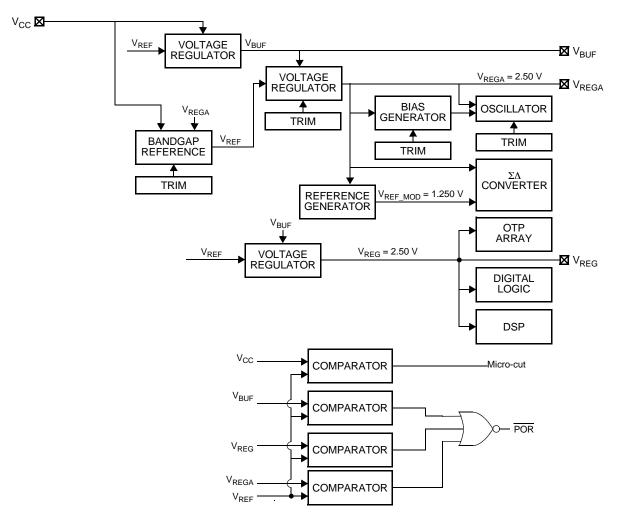
Figure 8. Voltage Regulation and Monitoring
