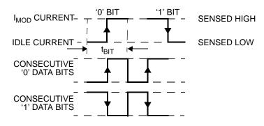
Figure 29. Manchester 2 Data Bit Encoding
