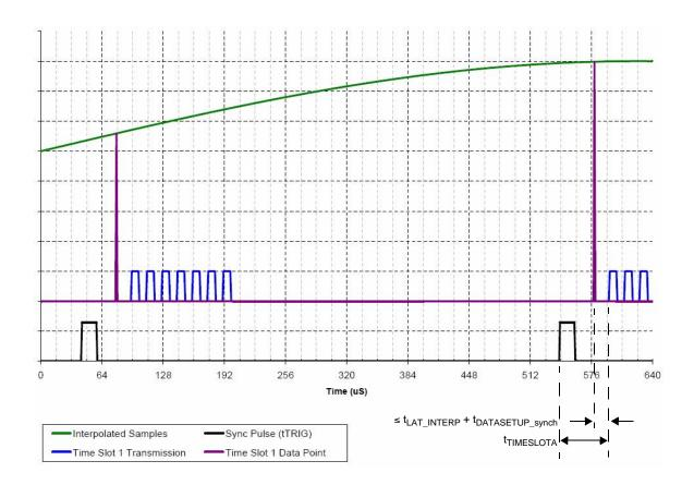
Figure 36. Synchronous Sampling Mode with Minimum Latency
