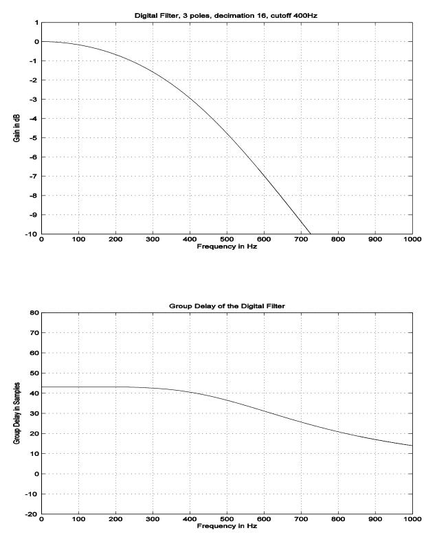
Figure 18. Low-Pass Filter Characteristics:  $f_{C}$  = 400 Hz, 3-Pole,  $t_{S}$  = 16  $\mu s$
