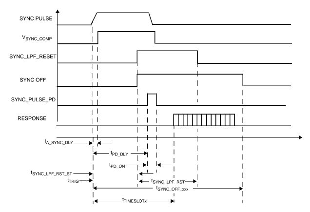
Figure 28. Synchronization Pulse Detection Timing
