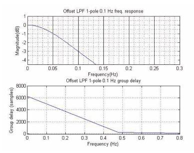
Figure 21. 0.1 Hz Offset Cancellation Low Pass Filter Characteristics
