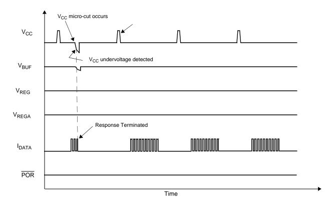
Figure 9. V<sub>CC</sub> Micro-Cut Response
