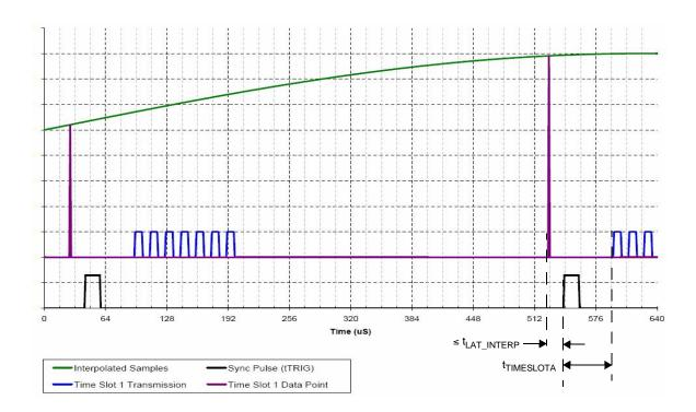
Figure 35. Simultaneous Sampling Mode
