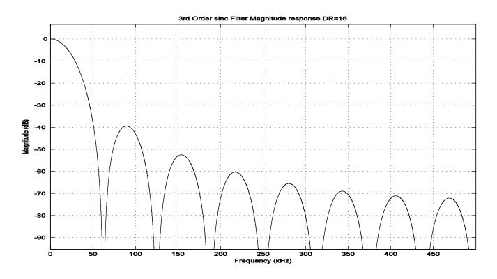
Figure 16. Sinc Filter Response, t\_{S} = 16  $\mu s$
