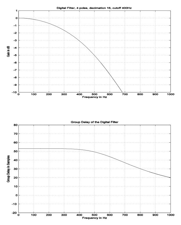
Figure 17. Low-Pass Filter Characteristics:  $f_{C}$  = 400 Hz, 4-Pole,  $t_{S}$  = 16  $\mu s$
