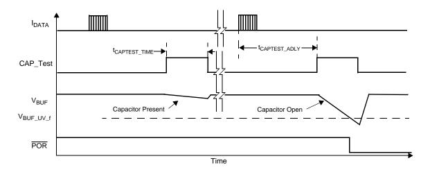
Figure 10. V<sub>BUF</sub> Capacitor Monitor - Asynchronous Mode
