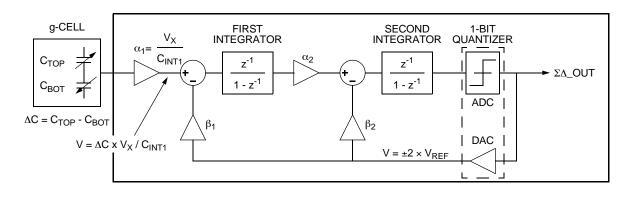
Figure 14.  $\Sigma\Delta$  Converter Block Diagram
