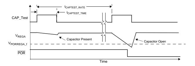
Figure 13. V<sub>REGA</sub> Capacitor Monitor
