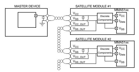
Figure 25. PSI5 Satellite Interface Diagram
