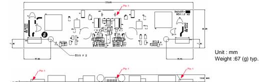
Note: Please use plastic screw in case of a non-insulating mounting base!
