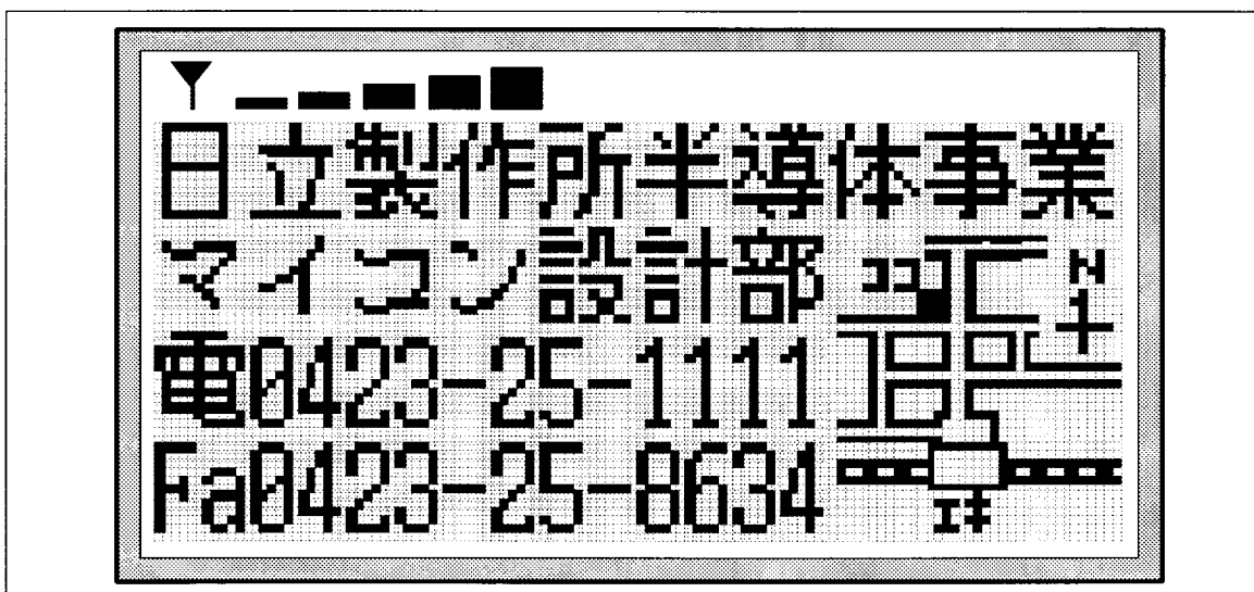
Figure 1 Combined Display of 4-line x 10-character Kanji and Graphics
