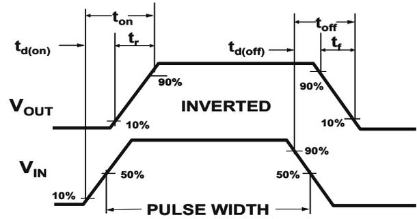
Figure 2:Switching Waveforms
