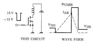
$$\begin{array}{l} T_{ch}=25^{\circ}C~(Initial)\\ Peak~I_{AR}=-3.5~A,~R_{G}=25~\Omega~~E_{AS}=\frac{1}{2}~\cdot L~\cdot I^{2}~\cdot (~\frac{B_{VDSS}}{B_{VDSS}-V_{DD}})\\ V_{DD}=-24~V,~L=1.48~mH \end{array}$$
