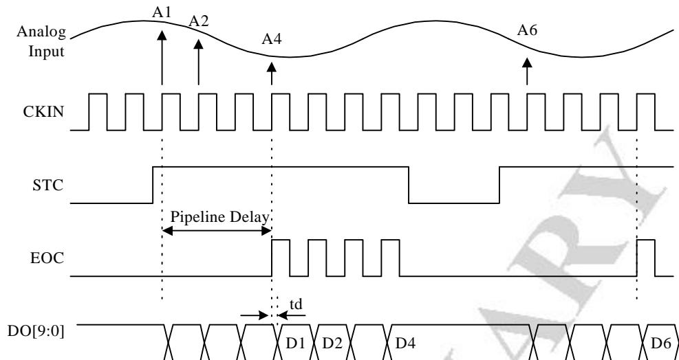
Output code of DO[9:0] is generated during STC (Start of Conversion) signal is just "HIGH". Otherwise, it keeps the current states.
