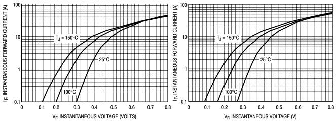
Figure 1. Maximum Forward Voltage, Per Leg
