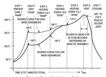
Figure 11. Typical Solder Heating Profile
