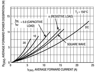
Figure 8. Current Derating, Free Air
