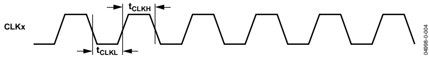
Figure 4. CLK Switching Characteristics (x = A, B, C, D for Individual Input Ports)
