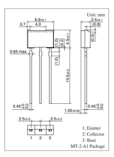
Note) \*: Copper plate at the collector is more than 1 cm<sup>2</sup> in area, 1.7 mm in thickness
