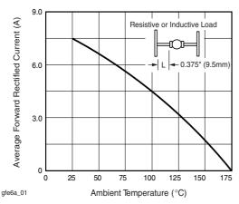
Figure 1. Maximum Forward Current Derating Curve
