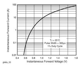
Figure 3. Typical Instantaneous Forward Characteristics
