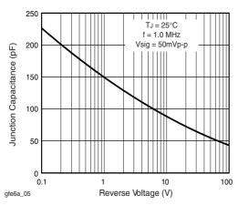
Figure 5. Typical Junction Capacitance
