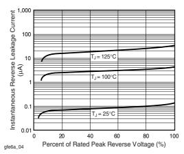
Figure 4. Typical Reverse Leakage Characteristics
