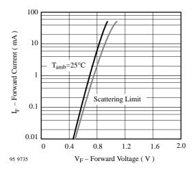
Figure 1. Forward Current vs. Forward Voltage
