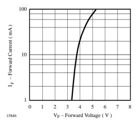
Figure 4. Forward Current vs. Forward Voltage
