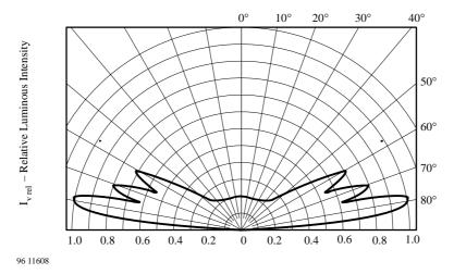
Figure 3. Rel. Luminous Intensity vs. Angular Displacement
