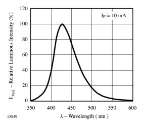
Figure 7. Relative Luminous Intensity vs. Wavelength
