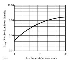
Figure 6. Relative Luminous Flux vs. Forward Current
