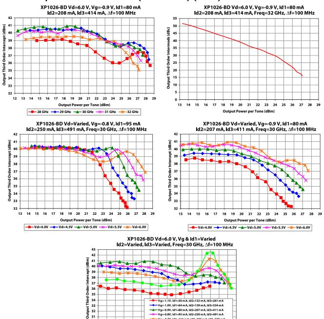
Note [1] Measurements - On-Wafer Output Power data has been taken using bias conditions as shown. Measurements are referenced 150 um in from RF In/Out pad edge. For optimum performance Mimix T-pad transition and tuned output matching network is recommended. For additional information see the Mimix "T-Pad Transition" application note. Contact technical sales for output matching network information.
