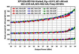
**Note** [1] **Measurements** – On-Wafer Output Power data has been taken using bias conditions as shown. Measurements are referenced 150 um in from RF In/Out pad edge. For optimum performance Mimix T-pad transition and tuned output matching network is recommended. For additional information see the Mimix "T-Pad Transition" application note. Contact technical sales for output matching network information.
