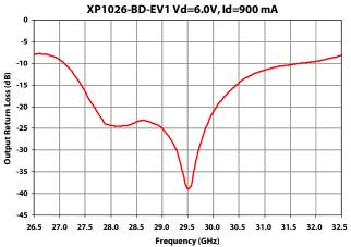
**Note [1] Measurements** – Test Fixture data includes all bond wire parasitics, uncompensated RF In/Out Mimix T-Pad transitions and RF ceramic circuit losses. For Gain and Output Power curves RF In/Out circuit losses have been removed.
