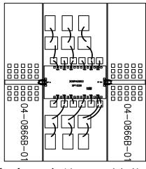
**Layout for reference only** – It is recommended to bias output stage from both sides.
