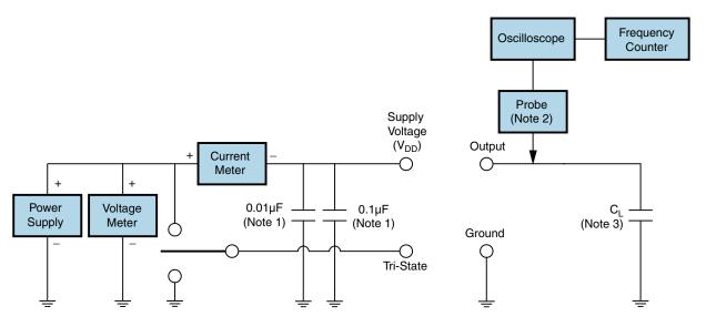
Note 1: An external 0.01µF ceramic bypass capacitor in parallel with a 0.1µF high frequency ceramic bypass capacitor close (less than 2mm) to the package ground and supply voltage pin is required.
